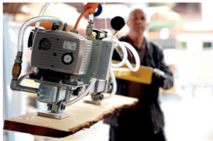
VacuWood VW-250KG For stacking wooden planks after a dividing saw.
