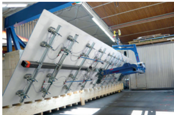
VacuGiant VG-180E-1500KG With balancing suspension and forklift shoes for turning plastic panels with dimensions of up to 16,000 x 3,500 x 10 mm
