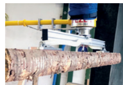
Suction pads for long goods With a reinforced longitudinal beam design for handling long goods up to 6,000 mm.
