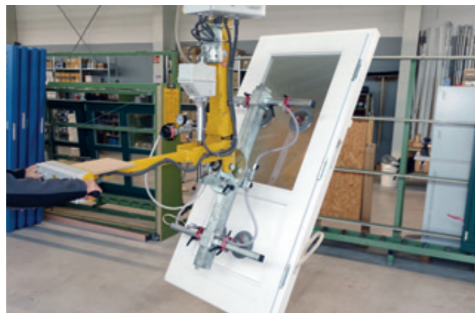
VacuBoy VB-90E-180-125KG With electric tilt drive and manual turning device in the production of window and door components
