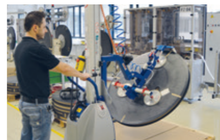
MobiliftMini ML-100KG-2000 With integrated vacuum technology and electrical slewing unit for coil units
