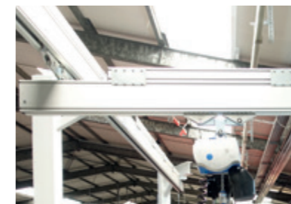
Bearer duplication In the case of very long gantry bridges, these can be reinforced by doubling the profile and thus moving higher loads
