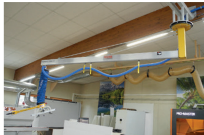
DSK-3500-100KG With 360° slewing range for loading a CNC machine
