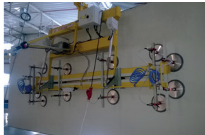
VacuBoySystem VBS-90E-1500KG For tilting of coated panels
