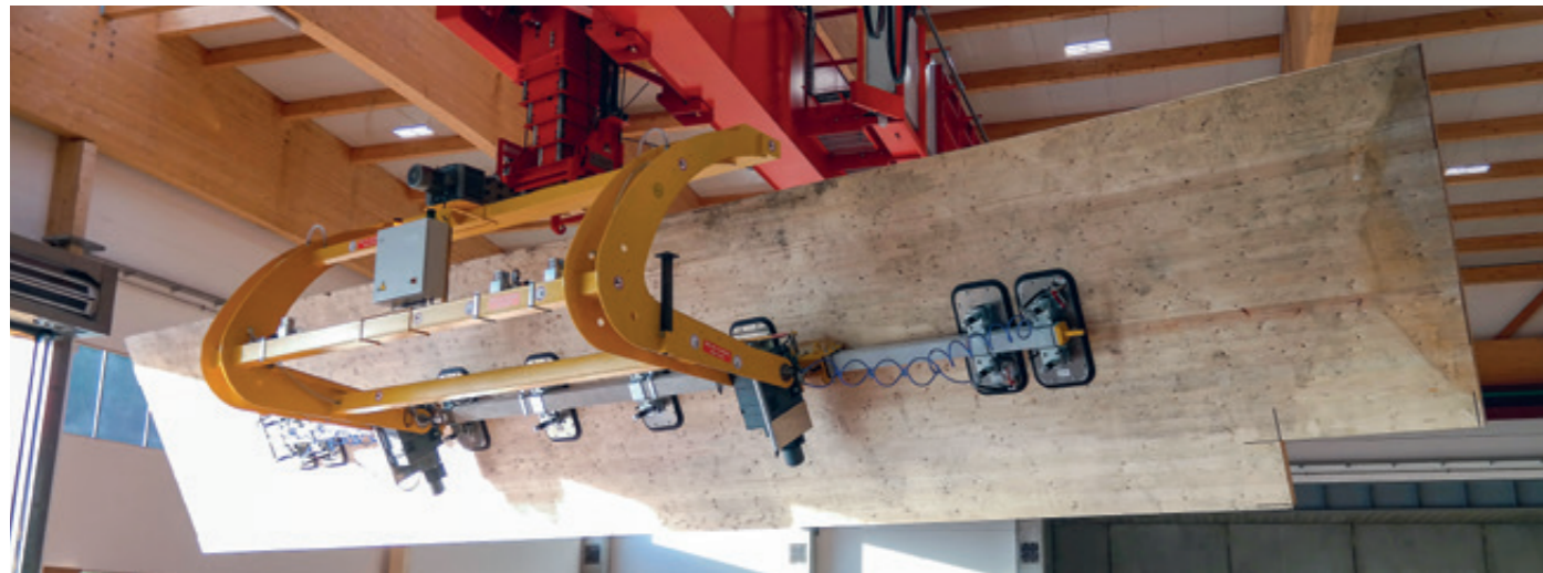
VacuGiant VG-180E-5000KG Turning solid wood panels up to 12,000 x 3,500 x 100 mm
