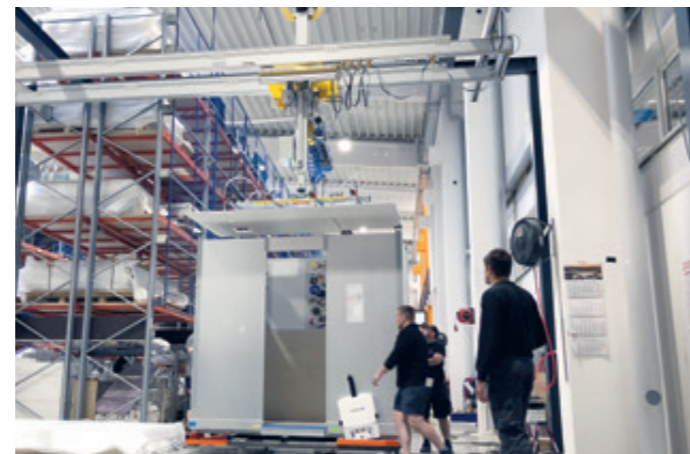
Liffix LF-ET-80KG Rigid double-telescopic lifting system for handling cover elements in final assembly
