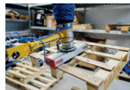
Flat gripper With surface suction pad and integrated ejector.
