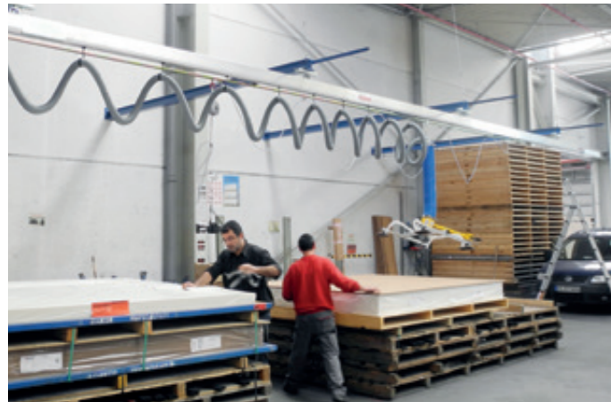
HBS-ES-125KG-12000 Single rail crane for moving panel material
