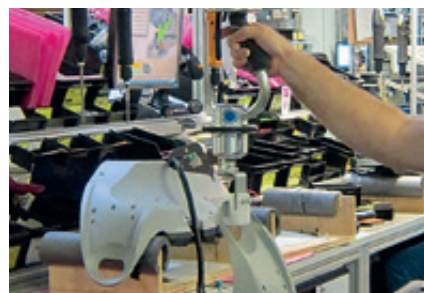
Mechanical lower gripper with compensating valve for handling loads by reaching under.
