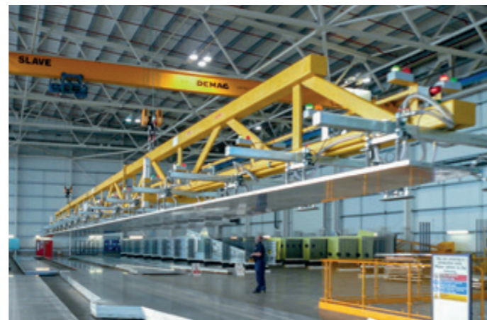
VacuGiant VG-5000KG Transport of blank aluminum panels up to 36,000 mm long for the wing production of the Airbus A380
