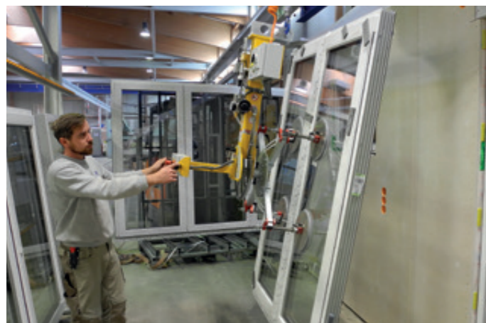
VacuBoy VB-VERT-180-125KG Handling of window components in pre-assembly
