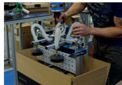
Combi-gripper And the subsequent restacking of the packed boxes using a quadruple suction pad.
