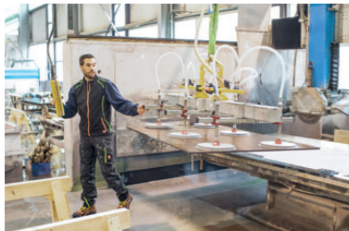
VacuBoy VB-250KG Handling of wet stone slabs
