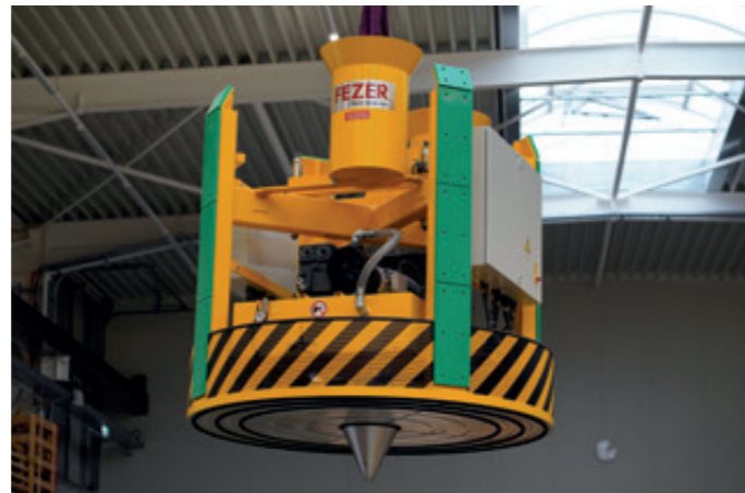
VacuCoilPaper VCP-4000KG In the automatic warehouse with 3 suction chambers, automatic chamber recognition and centering mandrel
