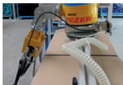
Rapid ventilation Additional ventilation valve for faster ventilation and detachment with dense workpieces. Simple operation via hand lever.
