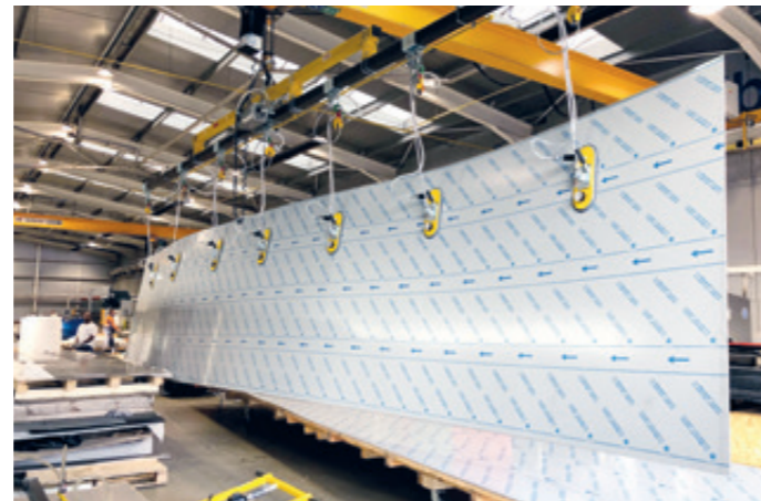
VacuBoyVario VBV-250KG Setting up plastic panels with a length of up to 8,000 mm
