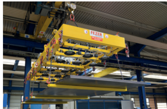
VacuGiant VG-5000KG-TEL Combination traverse for the transport of individual sheets with vacuum as well as complete bundles of sheets
