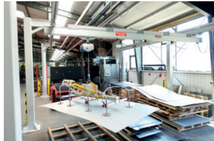
HBS-EB-500KG-12000x6000 Single beam crane system with reinforced gantry for higher loads
