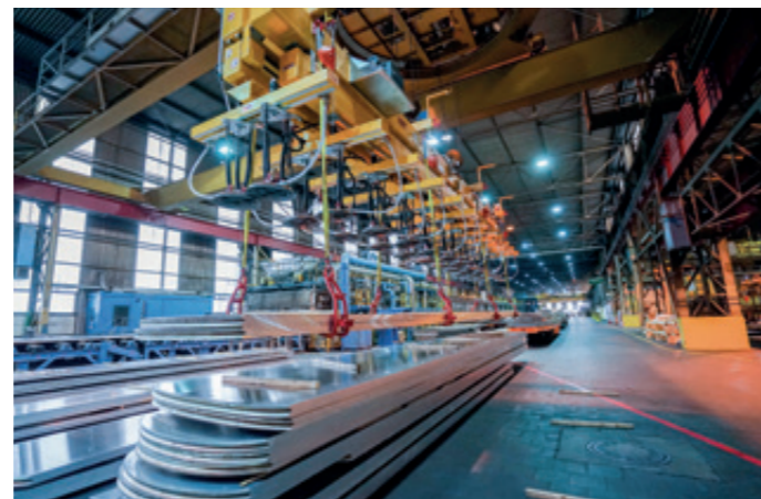
VacuGiant VG-12000KG-TEL Electrical extensible vacuum traverse with package grippers for picking up several sheets at the same time
