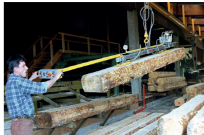
VacuWood VW-500KG For feeding logs to a lattice saw.
