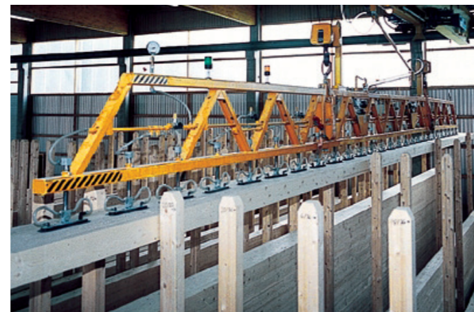
VacuWood VWLB-750KG For order picking of 16,000 mm long pieces of wood in a stanchion store
