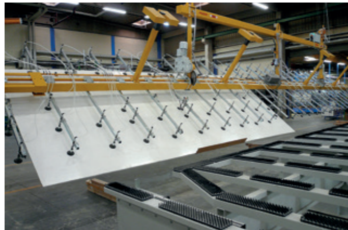
VacuGiant VG-90E-2500KG For truck side parts up to 13,500 mm in length
