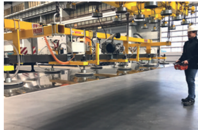
VacuBoySystem VBS-2500kg With 4-point suspension for sheets up to 8,000x2,500x30 mm
