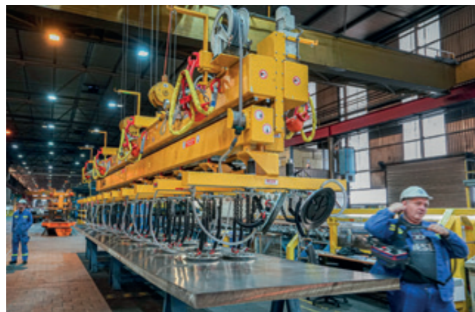
VacuGiant VG-12000KG-TEL Electrically extendable vacuum traverse for sheets from 8,000 - 14,000 mm with additional package grippers
