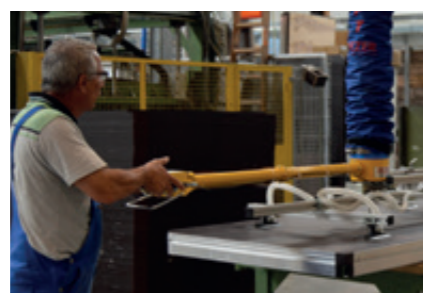
Rigid extension For safe operation of large-format workpieces.
