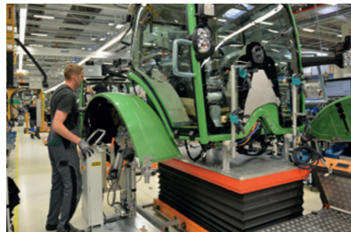
VacuStand VS-I-AL-FTS With ACCU module and electrical height and slewing adjustment
