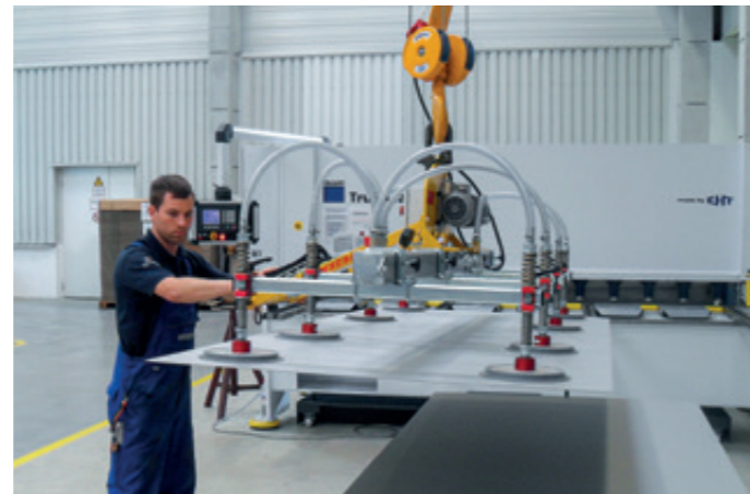
VacuBoy VB-750KG Handling of large format sheets
