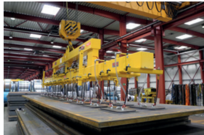
VacuGiant VG-25000KG With double-row suction pad arrangement for sheets up to 20000 x 3000 x 50 mm
