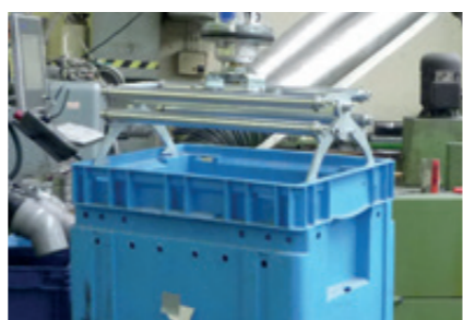
Box gripper Mechanical gripper with clamp gripper for handling boxes and containers.
