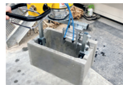
Pneumatic gripper With clamping device for moving hollow blocks.
