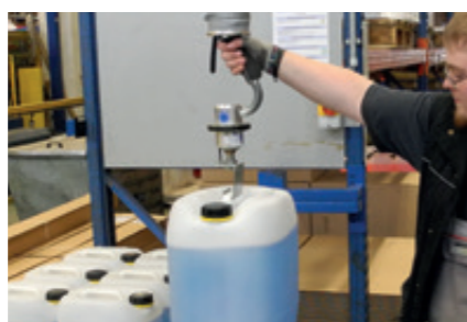
Canister gripper Mechanical bottom gripper for containers or canisters with handles or brackets.
