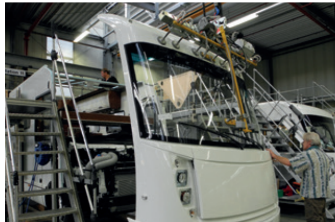
VacuBoy VB-VERT-125KG For the assembly of front glass panes
