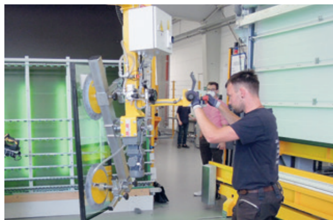
VacuBoy VB-VERT-180E-250KG With electric rotary drive in the production of multi-glazed window panes
