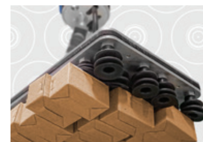
Multigripper Our Multigripper was specially developed for our VacuQuicklift tube lifter and can easily suction loads with different sizes and surface conditions. Even small crevices and cracks are no obstacle. The special feature of this innovation? The total of 40 built-in nozzles and bellows suction cups ensure optimum surface adaptation and ensure that the "false air" sucked in by unoccupied suction cups does not cause any significant loss of performance.
