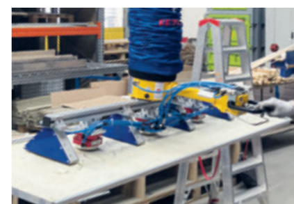
Combi-gripper With needle and magnetic gripper for handling insulating material and perforated sheets. Control via 2 pneumatic valves.
