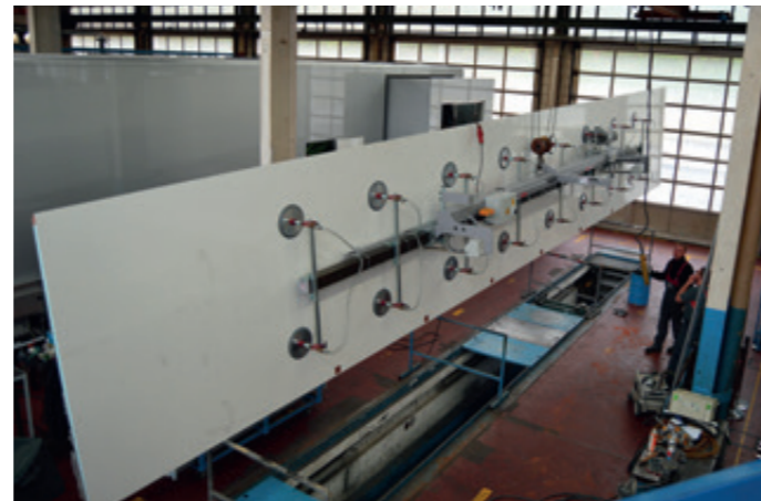
VacuBoySystem VBS-90E-1000kg For the assembly support of truck side parts up to 12,000 mm in length
