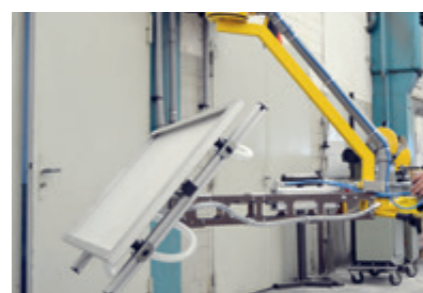
Pneumatic reversing unit Compact and robust, pneumatic device for reversing workpieces by 180°. The height of the turning bracket is adjusted to the workpiece size.
