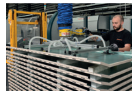
Sextuple suction pad For handling large and thin-walled sheet material.
