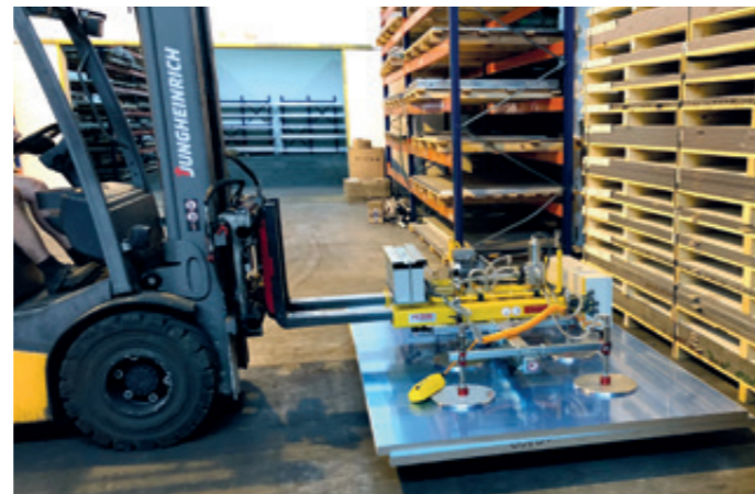
VacuBoyForker VBF-250KG-BATT With autonomously operating batteries for picking large-format metal sheets
