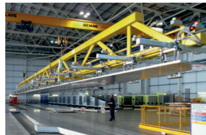
VacuGiant VG-5000KG For the transport of up to 36,000 mm long aluminum plates for the production of wing elements for the Airbus A380
