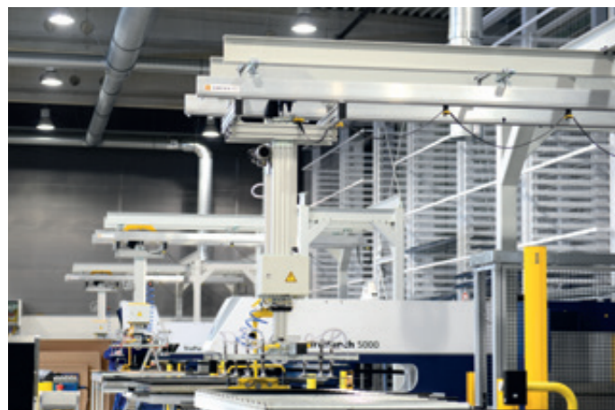
Liffix LF-DT-250KG Rigid lifting system with double telescope for handling steel plates
