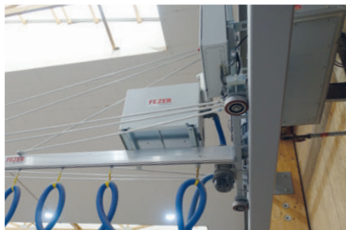
Wall mounted travelling crane WLK-120KG-44.000x7.000 with electrically movable jib (7,000 mm) with integrated collision prevention.
