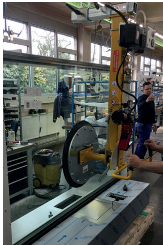
VacuBoy VB-VERT-180-125KG Handling of window components in the manufacturing process
