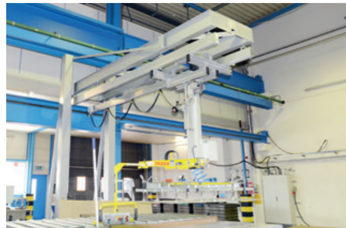
HBS-ZS-500KG-6000 Double rail crane with Liffix for loading sheet metal into a laser cutting system
