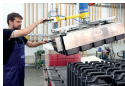
Canister grabber Pneumatically equipped clamping gripper for the simultaneous transfer of up to 20 canisters at once.
