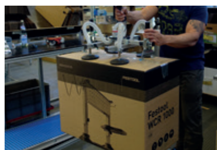
Combi-gripper With foldable lower grippers for packing racks in a box.
