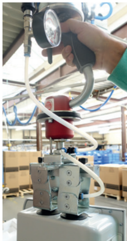
High vacuum gripper With pneumatic module, separate vacuum generator and manual slide valve for handling workpieces with small suction surfaces.
