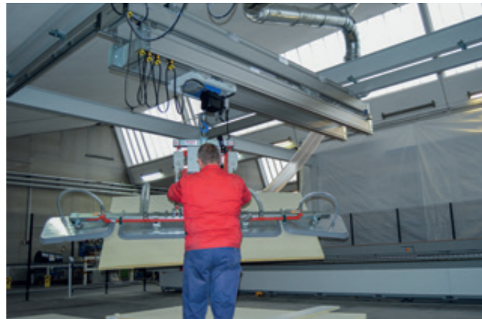
HBS-DB-500KG-8000x4000-TEL2000 Feeding of a CNC machining station via a telescopic double gantry
