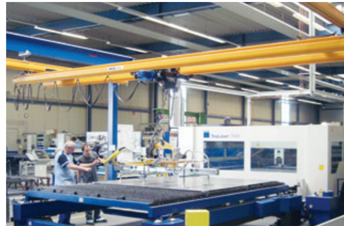
HBS-DB-800KG-6000x8000 Two beam crane for spanning a gantry length of 8,000 mm
