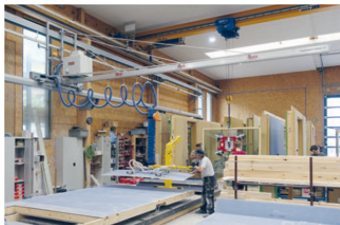
Wall mounted travelling crane WLK-80KG-36.000x7.500 for Fermacell, MDF and chipboards up to 3.000x1.250 mm
