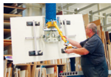
Pneumatic tilting unit Device via one or two pneumatic cylinders for tilting workpieces up to 150 kg.
