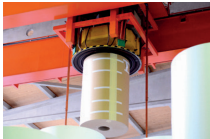
VacuCoilPaper VCP-6000KG In the automatic warehouse for paper rolls up to 2,500 mm in diameter and widths up to 2,750 mm
