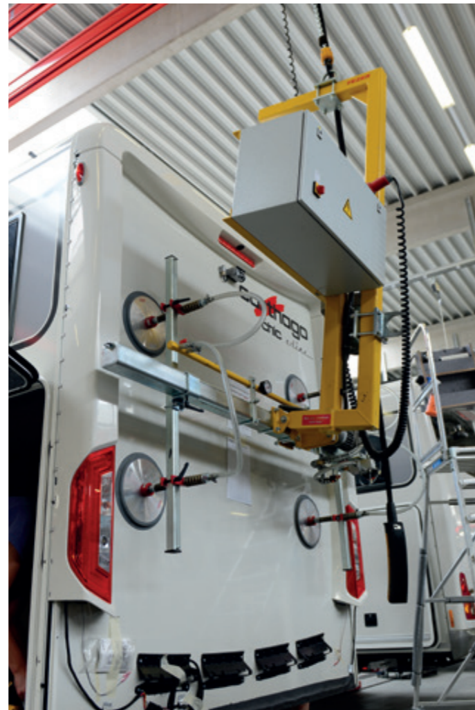
VacuBoy VB-VERT-250KG For the final assembly of rear walls in the mobile home industry
