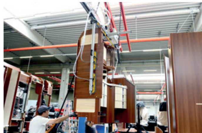
VacuBoyVario VBV-125KG Handling of completely prefabricated furniture parts in the final assembly
