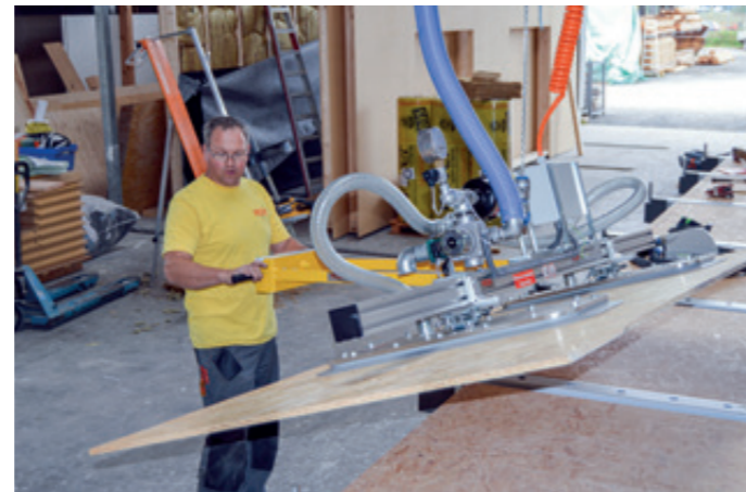
VacuPoro VP-500KG With separately installed blower for OSB panels
