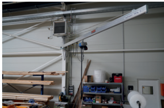
WSK-5000-100KG Clamped to a hall pillar in the packaging area
