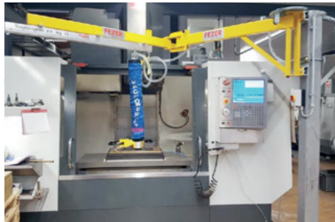
KSK-2500-2500-80KG For loading a processing machine
