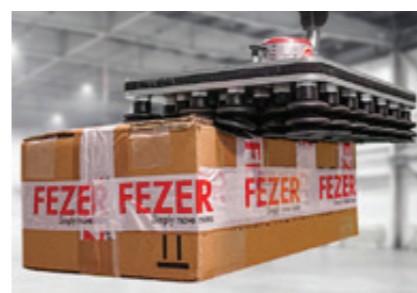
Multigripper Our Multigripper was specially developed for our VacuQuicklift tube lifter and can easily suction loads with different sizes and surface conditions. Even small crevices and cracks are no obstacle. The special feature of this innovation? The total of 40 built-in nozzles and bellows suction cups ensure optimum surface adaptation and ensure that the "false air" sucked in by unoccupied suction cups does not cause any significant loss of performance.
