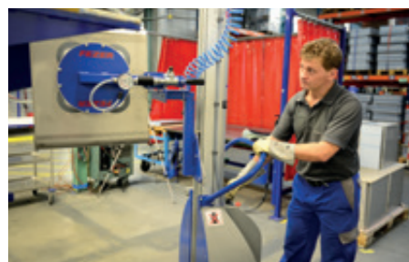
MobiliftMini ML-200-1500-100KG With integrated vacuum technology for handling metal containers
