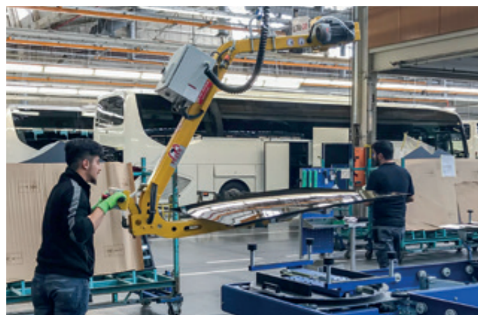
VacuBoy VB-180E-50KG In a low design via toothed rack for glass panes
