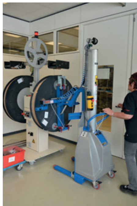
MobiliftMini ML-100KG-1500 For loading a coiler mandrel with copper coils
