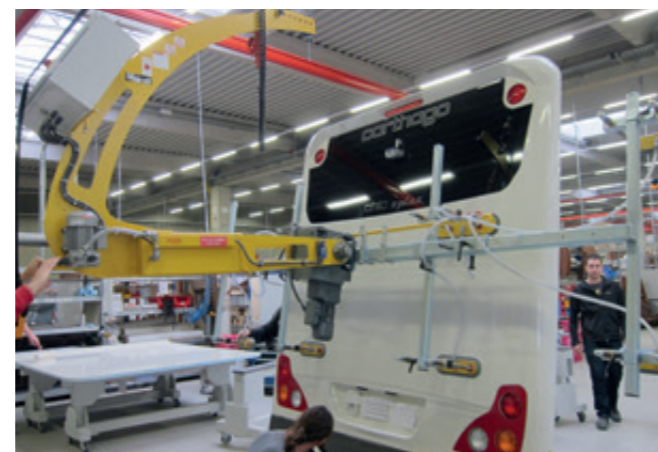
VacuBoy VB-180E-250KG For reversing and as an assembly aid for tail units for mobile homes
