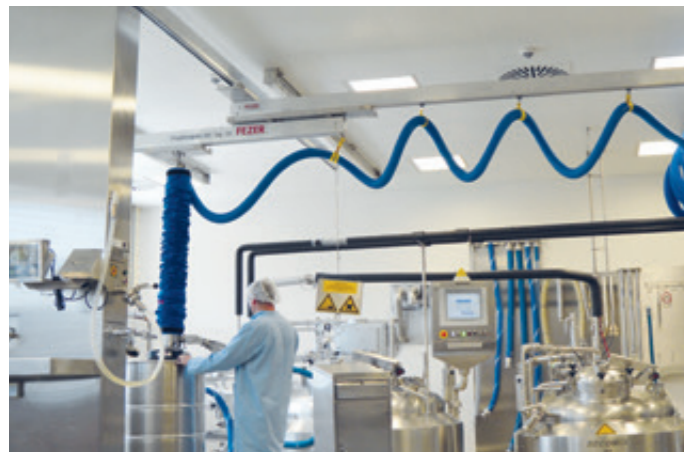
HBS-EB-80KG-10000x4000-TEL1500 Single beam crane system with telescoping single gantry
