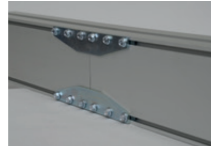
Profile connectors Stable and robust connecting plates enable crane rails of any length and stabilize the connection. The connection must be close to a hanger.
