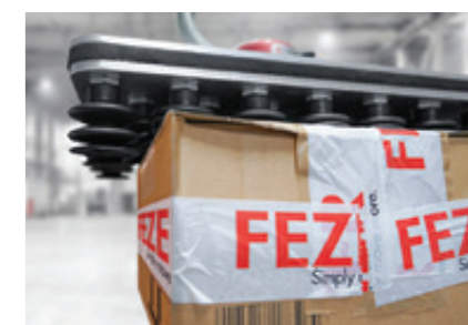
Multigripper Our Multigripper was specially developed for our VacuQuicklift tube lifter and can easily suction loads with different sizes and surface conditions. Even small crevices and cracks are no obstacle. The special feature of this innovation? The total of 40 built-in nozzles and bellows suction cups ensure optimum surface adaptation and ensure that the "false air" sucked in by unoccupied suction cups does not cause any significant loss of performance.
