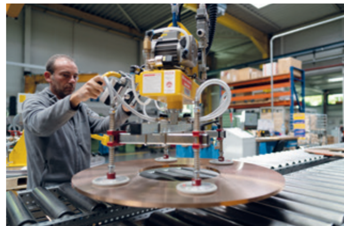
VacuBoyMini VBM-125KG handling of copper coils using a 4-fold attachment
