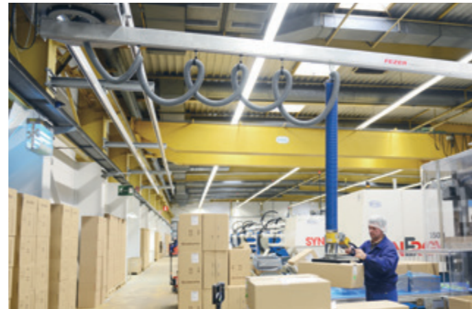
HBS-ZS-100KG-22000-SK-4000 Double rail crane with slewing ring for large-scale use of space
