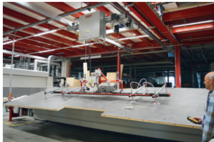
HBS-ZS-500KG-8000 Double rail crane with two chain hoists for handling floor components
