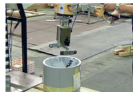
Pneumatic gripper With internal clamping jaws for moving coils.
