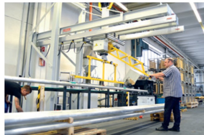
Liffix LF-ET-125KG Rigid lifting system with single telescope for pipe handling
