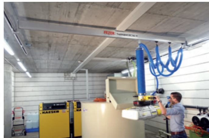
HBS-EBA-60KG-8000x4000 Single beam crane system with jacking for low overall height with maximum lifting utilization
