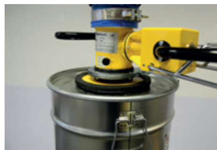
Single suction pads In round, flat or bellows design for drums, containers and small cardboard boxes.
