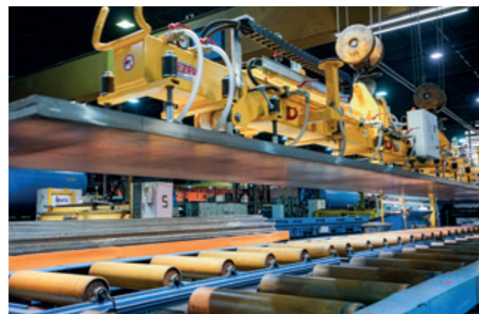
VacuGiant VG-12000KG-TEL In low and telescopic design for aluminum sheets up to 14,000x3,000x100 mm
