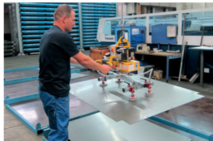
VacuBoyMini VBM-ACCU-125KG with quadruple suction pad for feeding a CNC system
