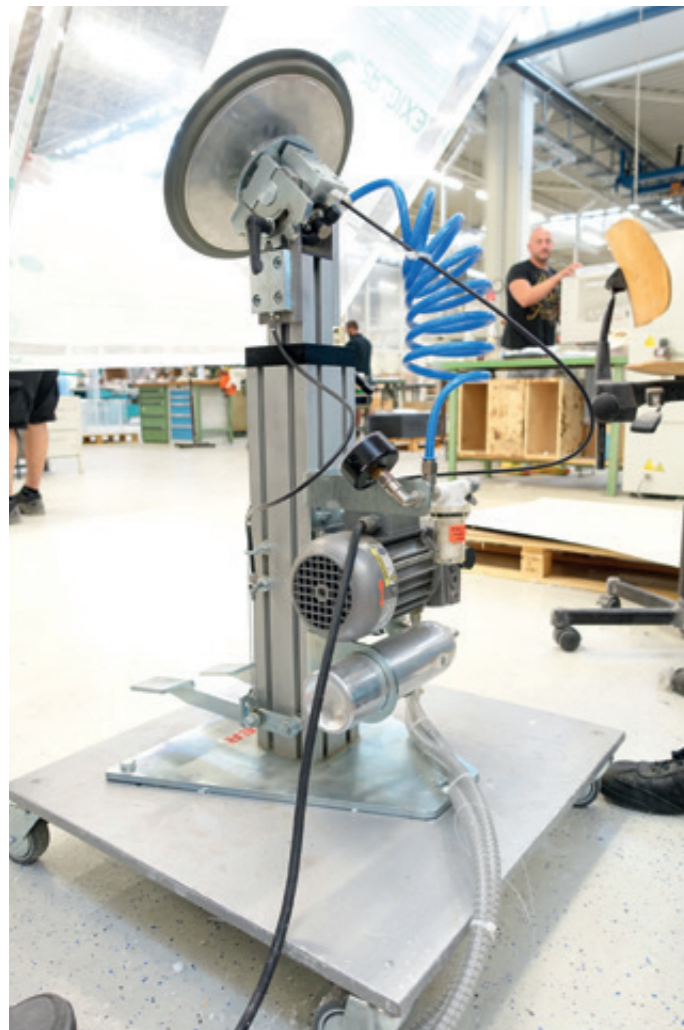
VacuStand VS-I-AL-FSRL290 Mounted on a mobile base plate with a single suction pad
