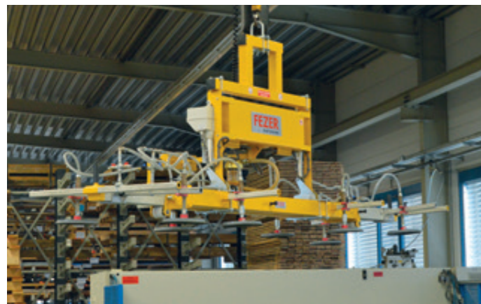
VacuBoySystem VBS-90E-750kg-TEL For sandwich components with lengths of 6,000-10,000 mm
