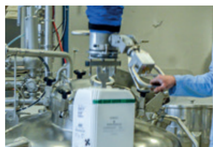
Canister grabber Simple hook gripper to grip under the canister tab with load balancing valve for vacuum control.
