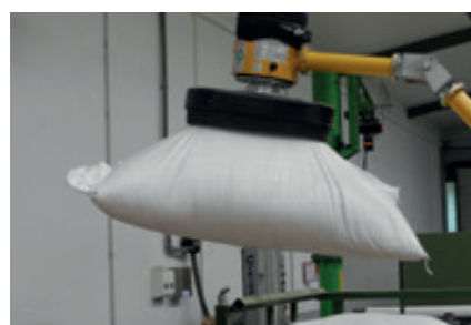
Sack suction cups Made of plastic with two sizes for smaller and larger paper and plastic bags.
