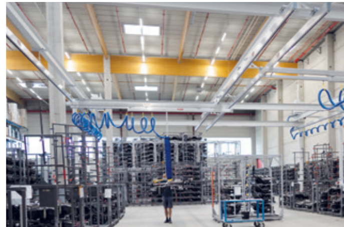
HBS-EB-80KG-12000x4000-TEL1500 Telescopic single gantries on a multi-girder crane system
