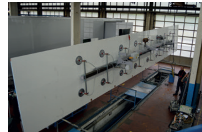
VacuGiant VG-90E-2500KG Electrically tiltable vacuum lifter for sandwich elements with a length of up to 12,000 mm
