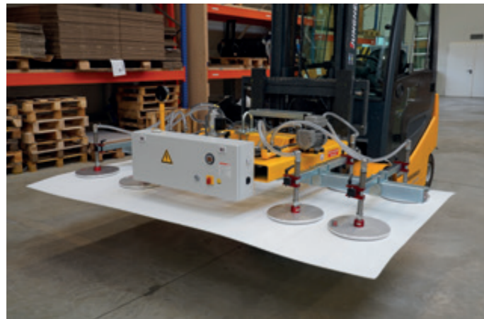
VacuBoyForker VBF-250KG-ACCU For large plastic panels up to 3,000x1,500 mm
