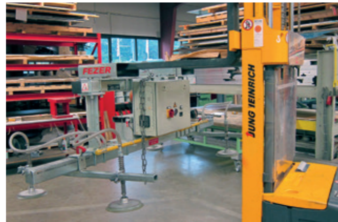
VacuBoyForker VB-250KG For moving sheet steel
