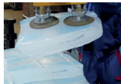
Bale suction pad With two flat suction pads with a special, reinforced rubber design.
