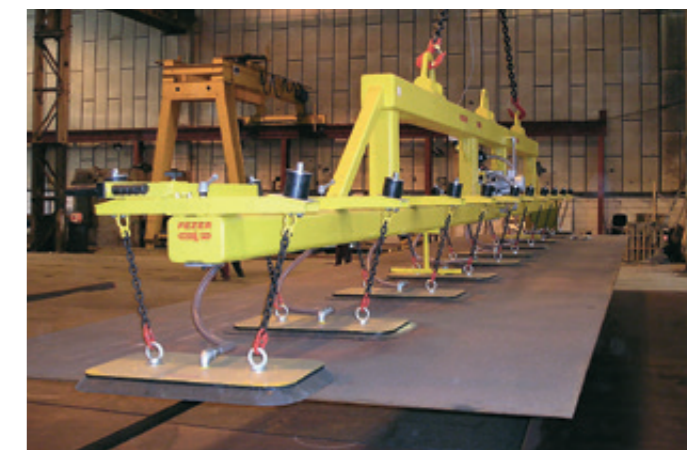
VacuGiant VG-12000KG With single-row suction plate arrangement for sheet steel up to 20,000 x 3,500 x 50 mm
