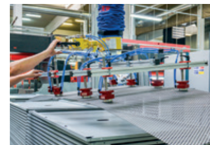
Magnetic gripper With pneumatic control for handling perforated sheets.
