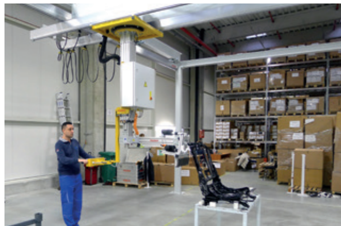
Liffix LF-ET-50KG Rigid lifting system with single telescope and load bearing for seat frames
