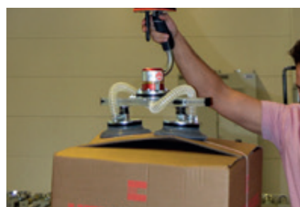
Cardboard gripper With two bellows suction cups for optimal adaptation to surface curvatures.
