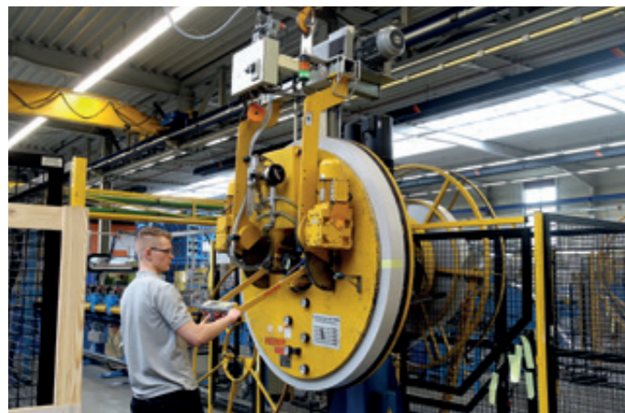
VacuCoil VC-90E-800KG For plastic coils in the production of roller shutter components
