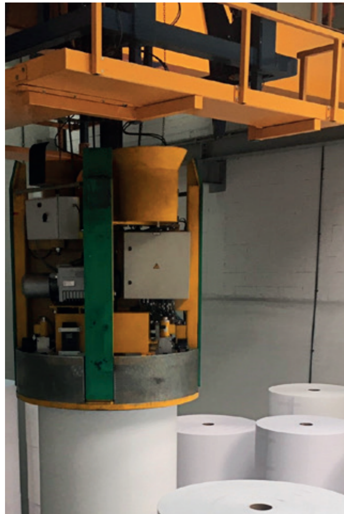
VacuCoilPaper VCP-5000KG In the automatic warehouse for paper rolls up to 2,000 mm in diameter and widths up to 2,000 mm
