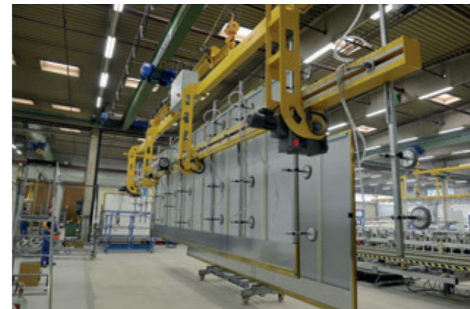
VacuGiant VG-VG90-2500KG Tilting traverse with slewing gear for the assembly support of truck bodies
