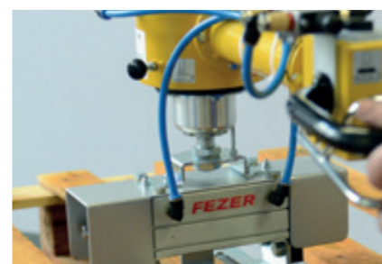
Balancing valve A compensating valve is available for the use of mechanical gripping devices, which takes over the automatic regulation of the vacuum.
