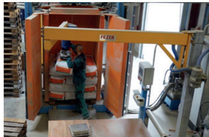
KSK-2500/2000-60KG With vacuum hose lifter for sack handling
