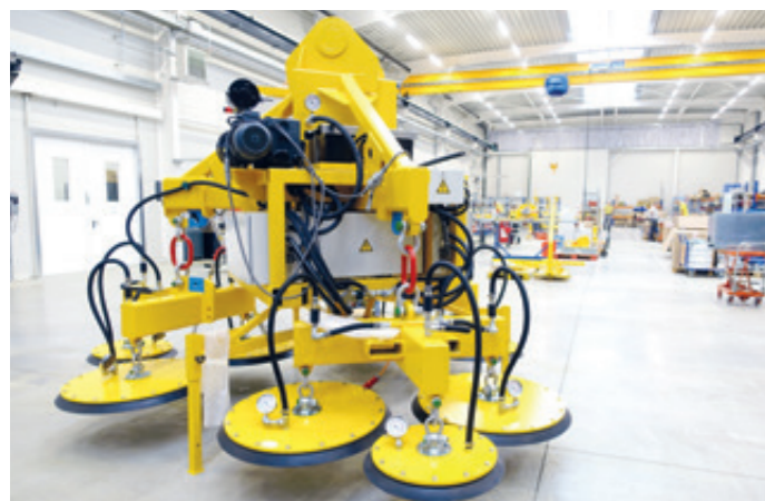
VacuGiant VG-18000KG Heavy-duty traverse for transporting glass blanks for telescope mirrors with a diameter of up to 6,000 mm
