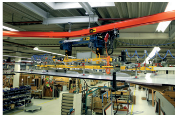
VacuBoySystem VBS-500kg In a flat design and with pivoting lower gripper as a safety precaution for transport over people
