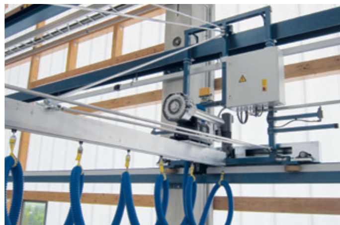
Wall mounted travelling crane WLK-100KG-68.000x7.000 with electrically movable jib (7,000 mm)
