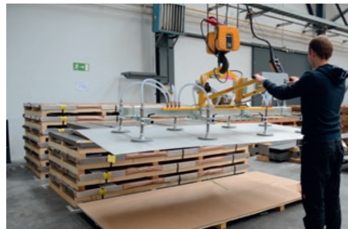
VacuBoy VB-1000KG Order picking of steel sheets
