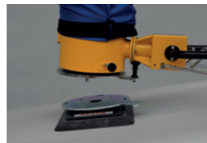
Quick-change coupling Facilitates the replacement of suction cups for various applications during ongoing operation.
