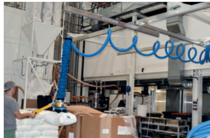
HBS-EB-60KG-6000x4000-TEL2500 Single beam crane system with telescoping single gantry for picking up sacks outside the working area
