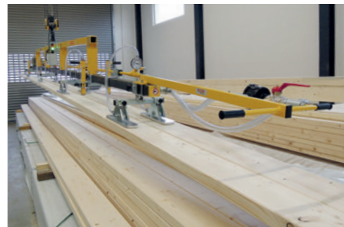
VacuWood VWLB-500 with double suction cups, simultaneous lifting of double-layer wood with a length of up to 12,000 mm possible
