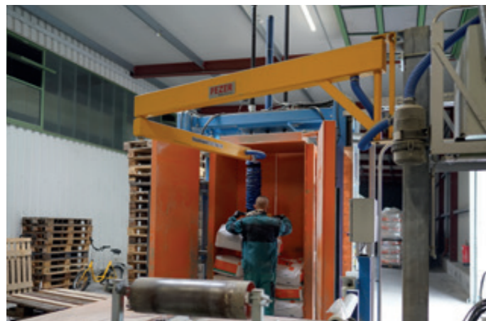
KSK-2500/2000-60KG For dipping into a sack system
