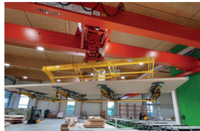
VacuGiant VG-180E-10000/2500KG With outrigger arms for turning 2,5000 kg wooden panels and horizontal transport of 10,000 kg concrete floor panels
