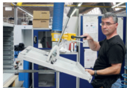
Manual tilting unit Simple and fast tilting device for tilting smaller workpieces up to approx. 35 kg.
