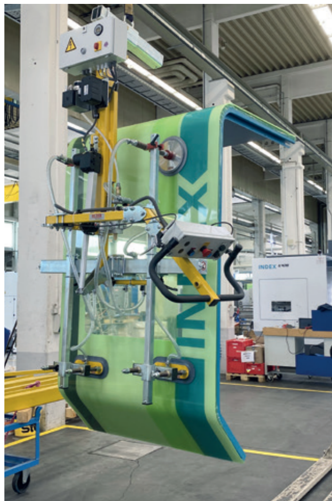
VacuBoy VB-90E-ACCU-125KG With double-jointed operating handle for the fitting of machine doors on CNC lathes
