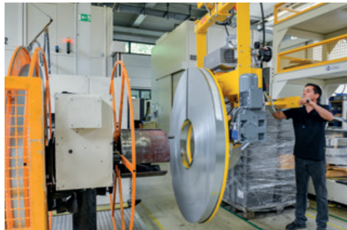
VacuCoil VC-90E-1000KG For aluminum coils up to 1,800 mm in diameter
