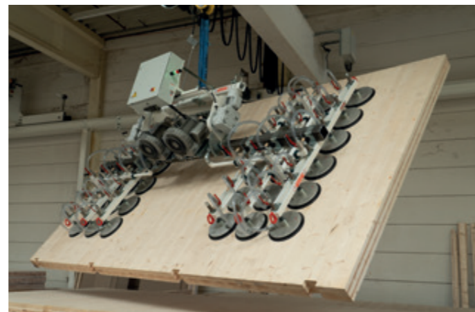
VacuGiant VG-90E-2500KG With 2 blower speeds in the final assembly of wooden containers
