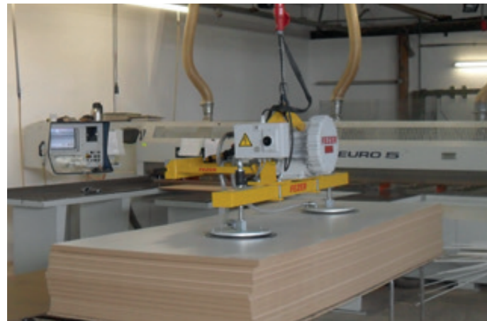
VacuPoro VP-250KG For handling raw and coated chipboard
