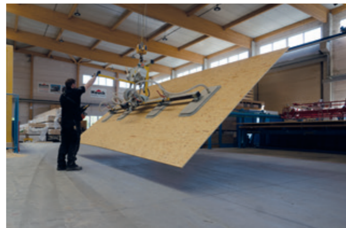
VacuPoro-90E-500KG For feeding a horizontal panel dividing saw
