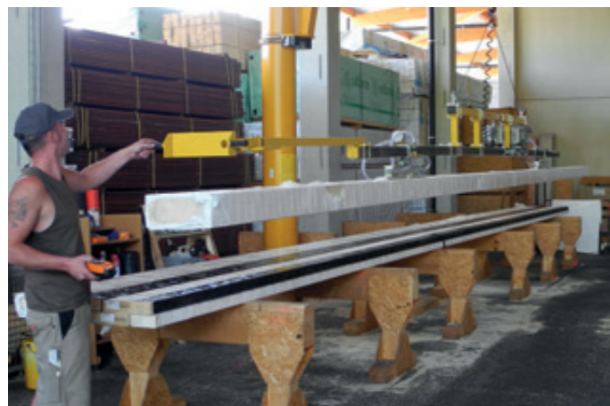
VacuWood VWLB-250 For laminated beams wrapped in film up to a length of 14,000 mm
