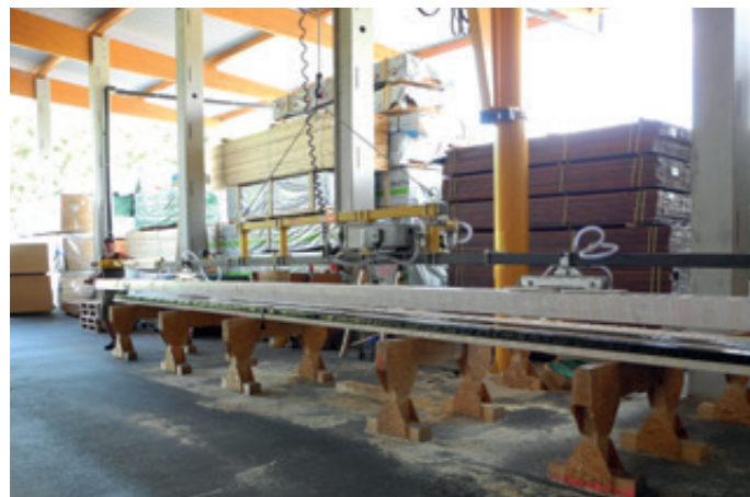
VacuWood VWLB-250KG For shifting logs up to 12,000 mm long
