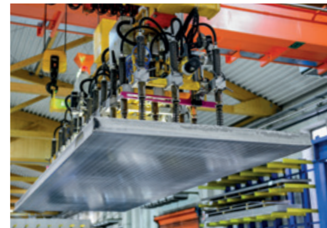
VacuGiant VG-6000KG Horizontal handling of aluminium plates 8000 mm in length in a rolling mill.
