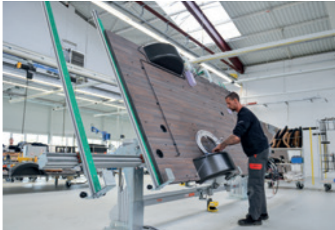
VacuStation SWS Stationary swivel station for the preassembly of mobile home floor elements.
