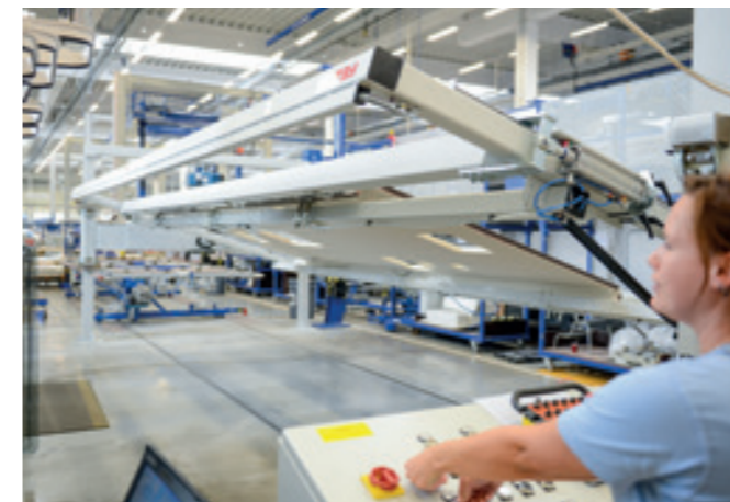
VacuStation SWS-360E-250KG Stationary turning system with pneumatic adjustment options for the preassembly of mobile home roofs.
