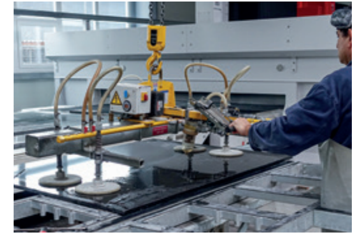
VacuBoy VB-250KG Loading stone slabs into a wet grinding machine using a battery-operated vacuum lifter.
