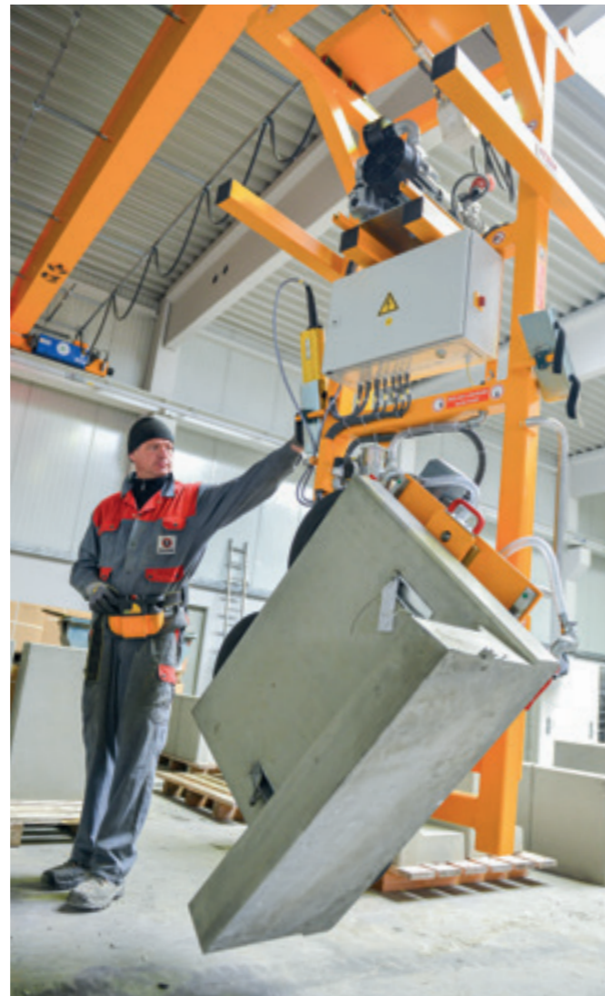
Vacuum Lifting Device VLM-VERT-180E-750KG Special vacuum lifter for turning L-shaped slabs for setting down safely.
