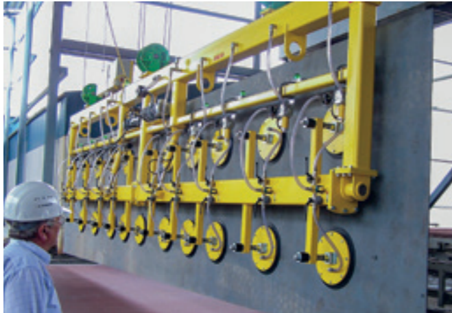
VacuGiant VG-90H-8000KG Hydraulically swivelling heavy-duty cross beam for sheet metal 8,000 mm in length in an upright bearing.
