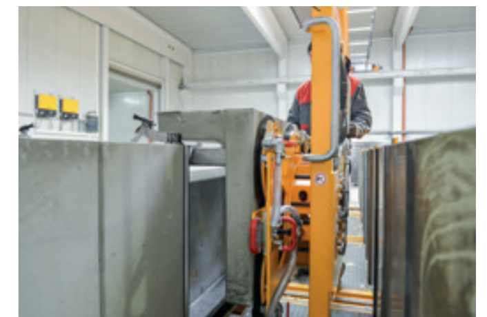
Vacuum Lifting Device VLM-VERT-180E-800KG Removing double L-shaped slab elements from the production mould.
