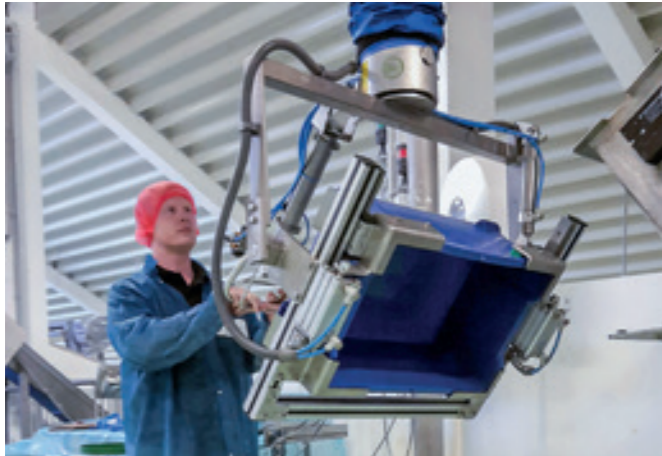
VacuPowerLift VPL140-50KG With pneumatic swivel unit for emptying canisters.
