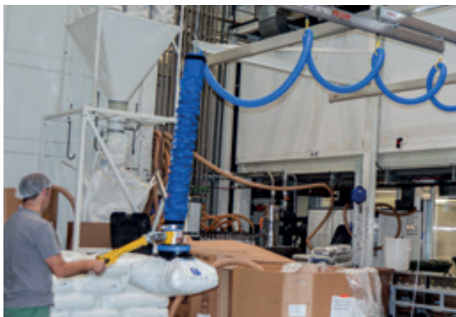
Aluminium overhead conveyor system HBS-EB-TEL-250KG With telescopic single bridge and tube lifter for handling bags.
