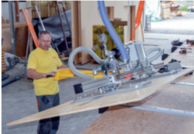
VacuPoro VP-250KG Loading a CNC machine with porous OSB plates.
