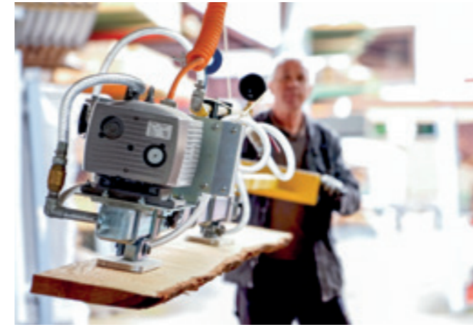
VacuWood VWB-250KG Handling rough-sawn wooden planks after a panel saw.
