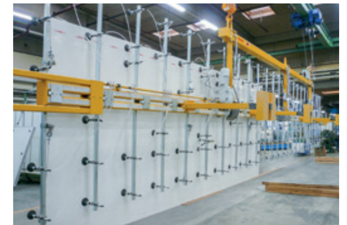
VacuGiant VG-90E-750KG Vacuum cross beam that can be swivelled on both sides for truck side parts up to 13,000 mm in length.
