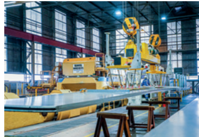
VacuGiant VG-TEL-4000KG Vacuum cross beam that can be pulled out by an electric motor for loading a stretching bench.
