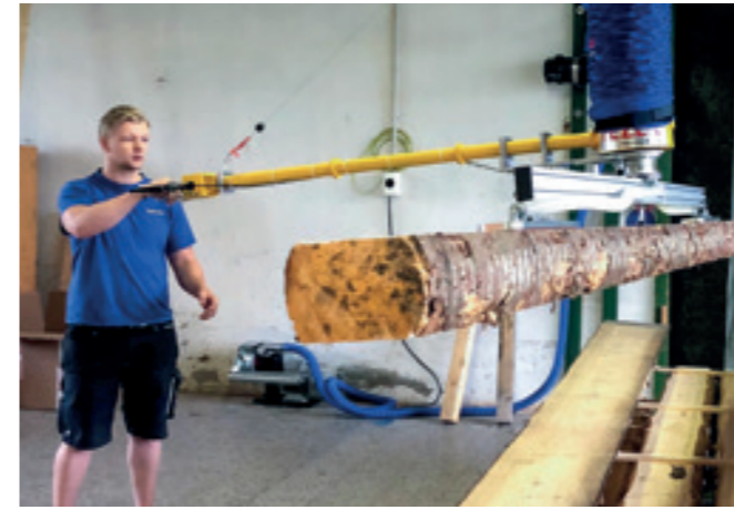
VacuPowerLift VPL-100KG For handling rough-sawn wooden planks.
