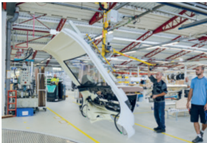
VacuBoy VB-90E-125KG Swivelling fully preassembled front elements
