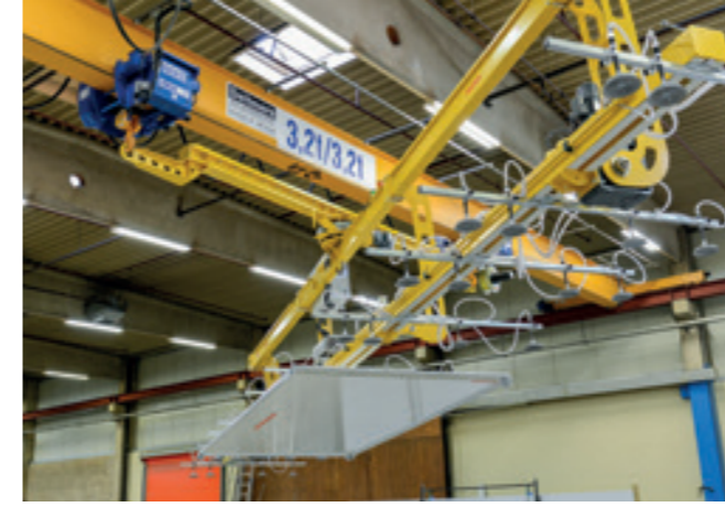
VacuGiant VG-90E-360E-2500KG Electrically swivelling and rotatable vacuum cross beam for handling truck side and roof elements.
