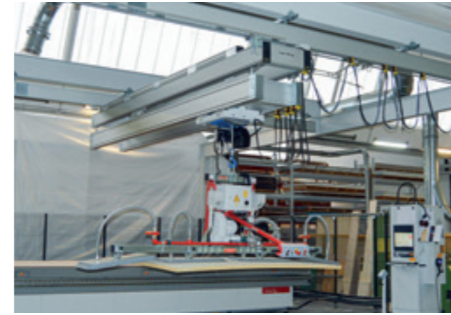
Aluminium overhead conveyor system HBS-DB-TEL-250KG with steel structure and telescopic double bridge in closed box shape.
