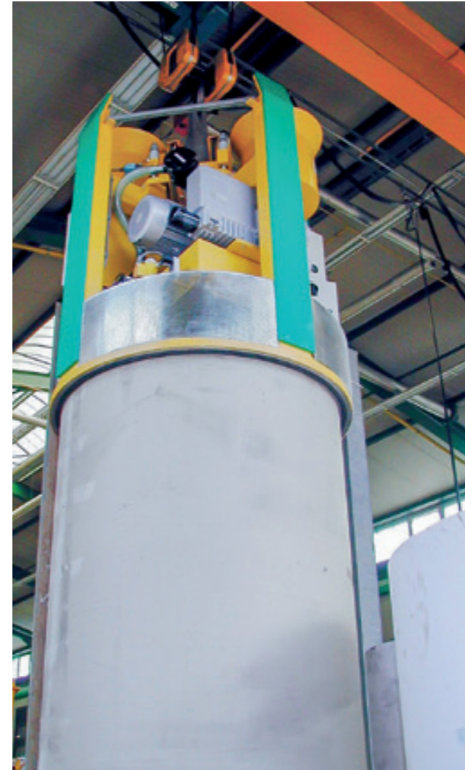
VacuCoilPaper VCP-4500KG-4SK Vacuum lifter for paper rolls up to 2,800 mm in height.
