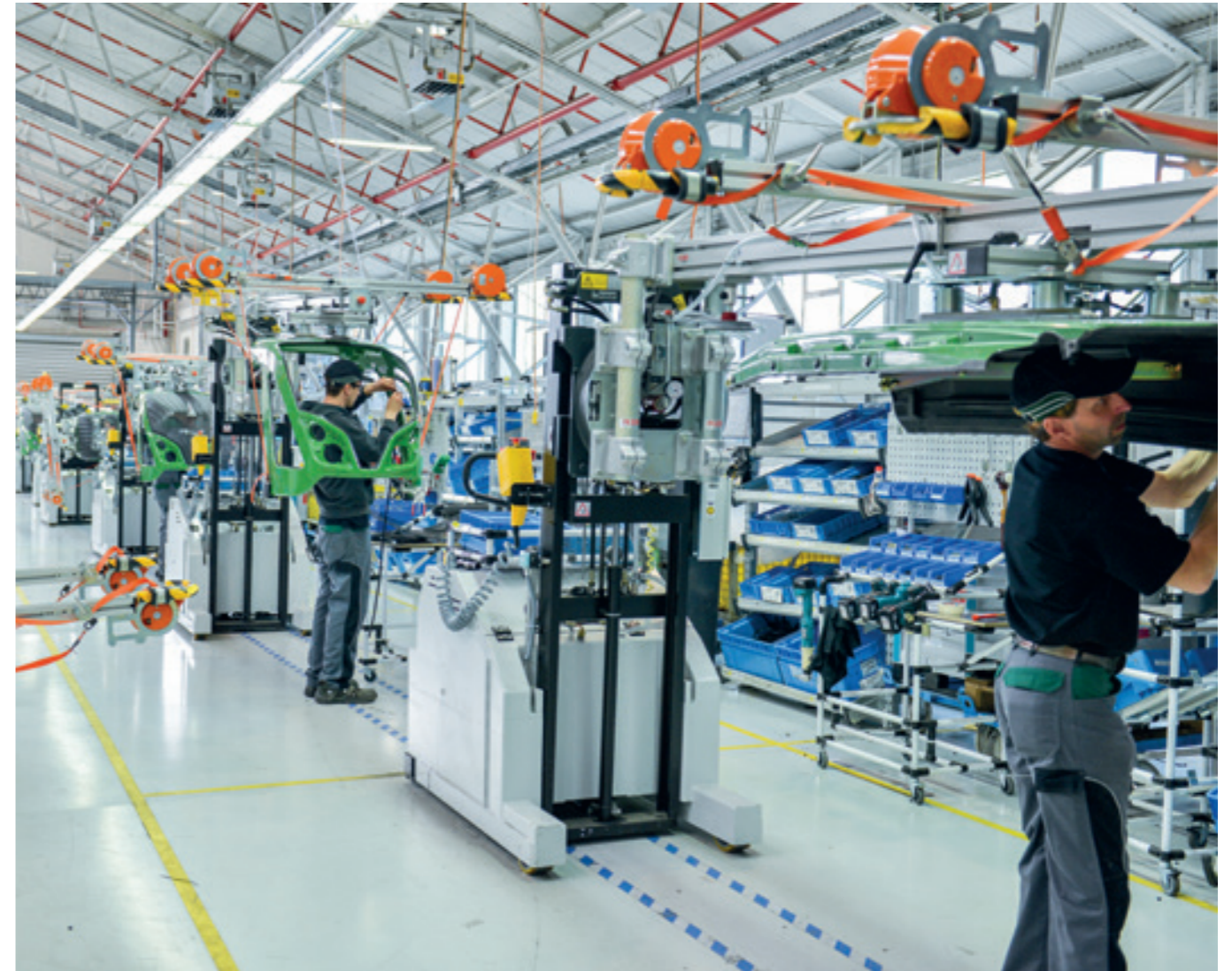
Mobilift ML-360E-125KG Mobile working stations in series production for the preassembly of complete hoods for tractors.
