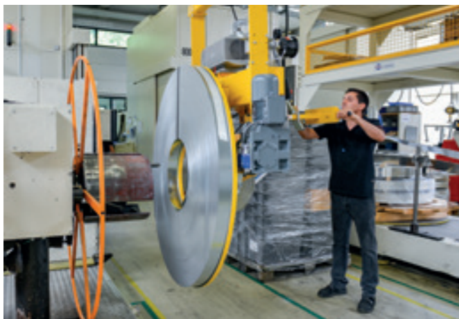
VacuCoil VC-90E-2000KG-5SK Swivelling vacuum lifting device for transferring slit strip rings to a decoiler mandrel.
