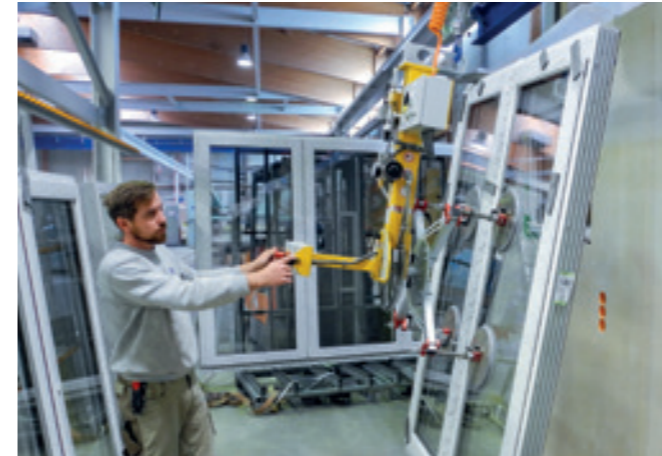
VacuBoyWindow-250KG Handling of window elements after final assembly.
