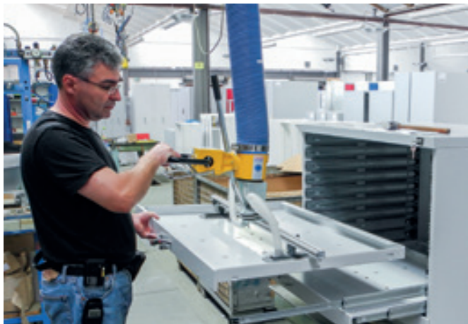
VacuPowerLift VPL-90M-45KG Tube lifter with mechanical tilting unit for assisting in the assembly of drawers.
