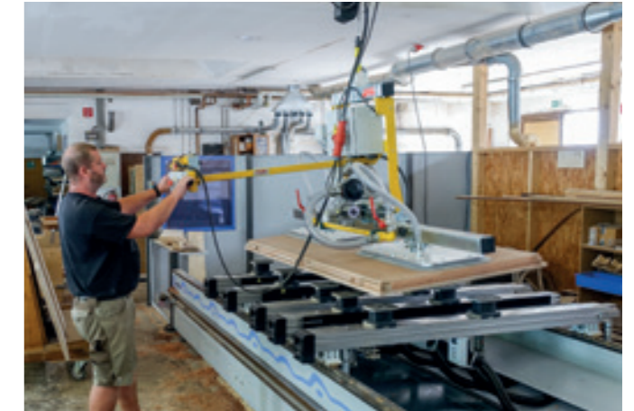
VacuPoro VP-90E-250KG Handling door elements on a CNC milling machine.
