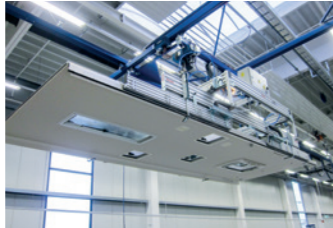
Vacuum Lifting Device VLM-250KG Handling of mobile home roofs following preassembly.
