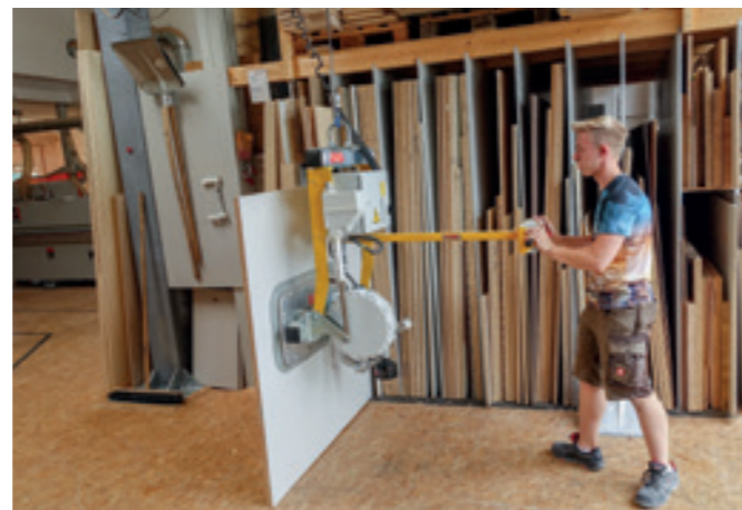
VacuPoro VP-90E-125KG Handling of wooden panels from an upright panel shelf system.
