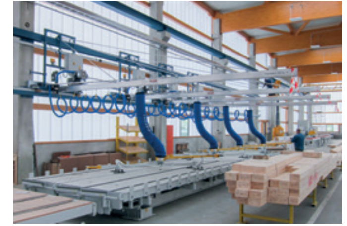
Aluminium overhead conveyor system HBS-4ALK-250KG Four jib crane systems, each with its own travel drive and moving blower for tube lifters.
