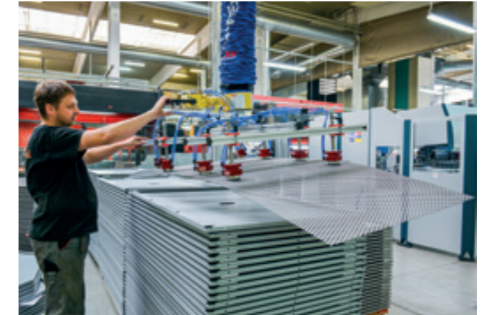
VacuPowerLift VPL-60KG Vacuum tube lifter with pneumatically controlled magnetic grippers for perforated sheets.
