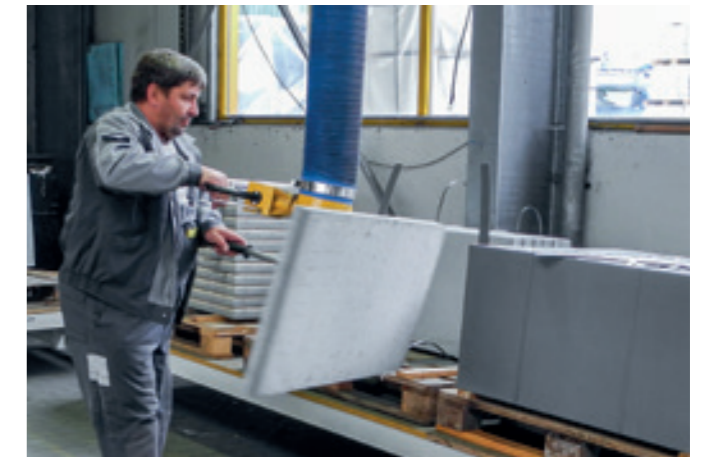
VauPowerLift VPL-90M-60KG Vacuum tube lifter with manual swivel unit for handling stone elements.
