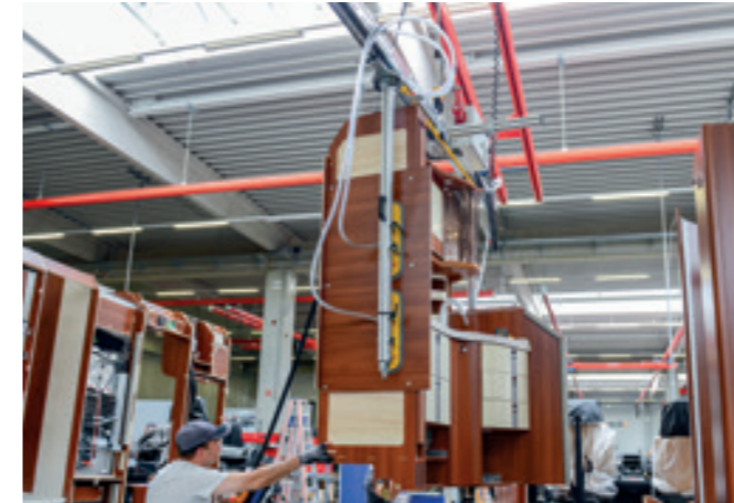
VacuBoyVario VBV-100KG Handling built-in cupboards in the preassembly of mobile home furnishings.
