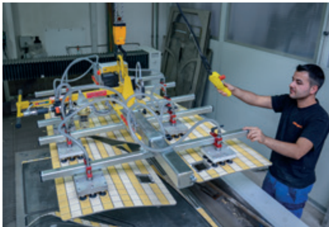
VacuBoy VB-ACCU-125KG Swivel-action vacuum lifting unit for handling pre-tiled wall elements.
