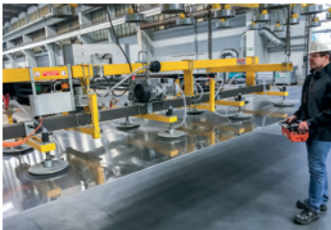
VacuBoySystem VBS-4000KG System cross beam traverse for horizontal handling of sheet metal up to 8,000 mm in length.
