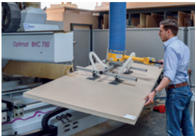
VacuPowerLift VPL-125KG Loading a CNC woodworking machine with porous wood elements
