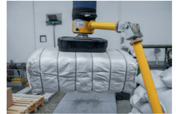
VacuPowerLift VPL-60KG Handling of plastic bags strapped with ropes.
