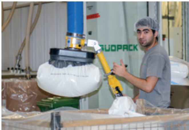
VacuPowerLift VPL-60KG Handling plastic bags.
