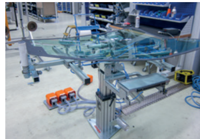
VacuStand VS-80KG Stationary working stand with pneumatic lifting and swivel unit for final assembly of tractor side windows.
