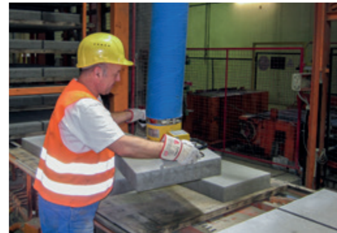
VauPowerLift VPL-60KG Vacuum tube lifter for handling paving stones.
