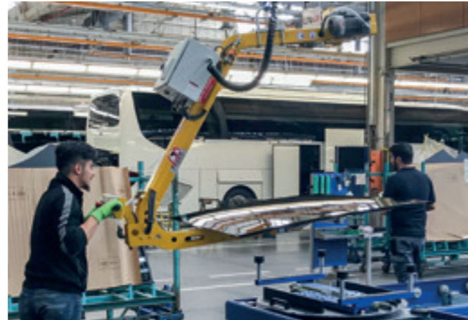
VacuBoy-180E-60KG Low-profile 180° turner for handling glass panes.
