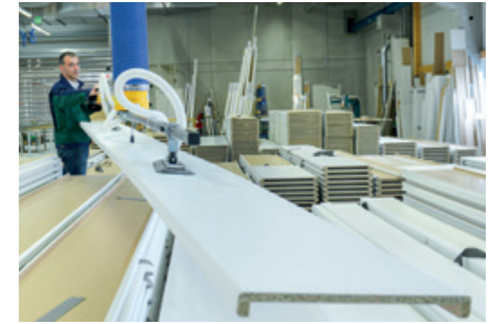
VacuPowerLift VPL-80KG Handling of coated wood worktops up to 6,000 mm in length.
