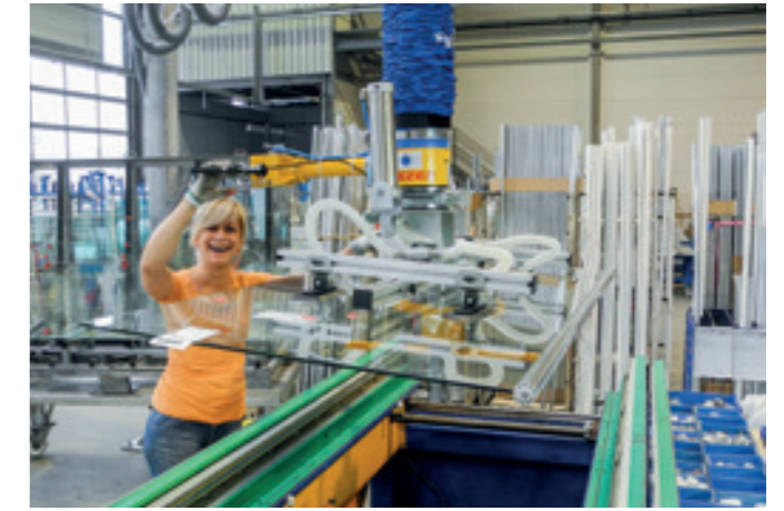
VacuPowerLift VPL180-90P-80KG Tube lifter with pneumatic swivel unit for glass panes.
