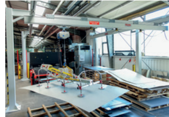
Aluminium overhead conveyor system HBS-DB-TEL-500KG with its own steel structure and reinforced bridge for increased load-bearing capacity.
