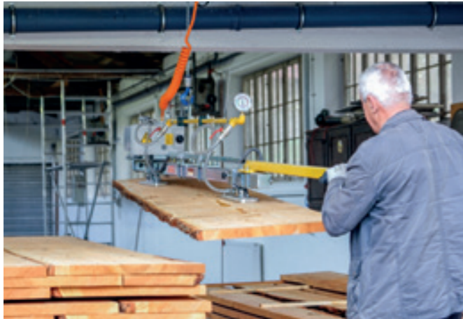
VacuWood VWB-250KG Moving rough-sawn wooden planks using a plank lifting device.
