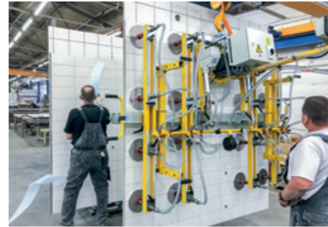
VacuBoy VB-90E-125KG Swivel-action vacuum lifting unit for handling pre-tiled wall elements.
