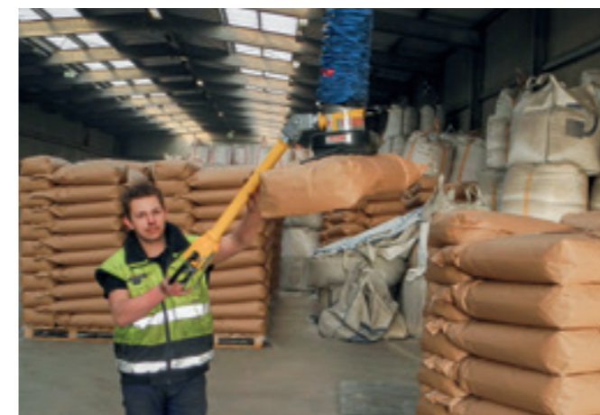
VacuPowerLift VPL-60KG Vacuum hose lifter for moving paper bags.
