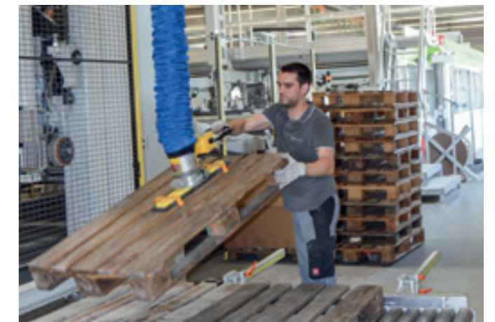
VacuPowerLift VPL-60KG With special suction gripper and centering unit for moving Euro pallets.
