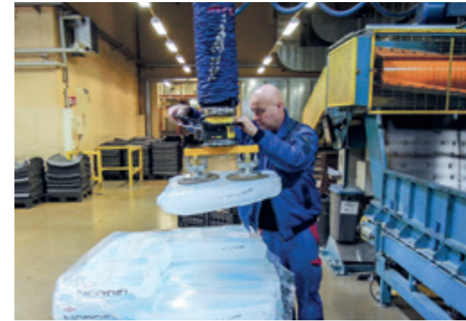
VacuPowerLift VPL-60KG With a special double suction gripper for handling rubber bales.
