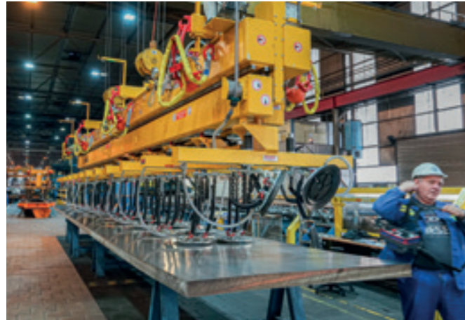
VacuGiant VG-TEL-6000KG Pull-out vacuum cross beam powered by an electric motor for sheet metal 6,000 - 14,000 mm in length.
