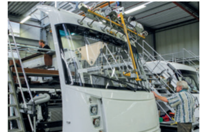
VacuBoy VB-VERT-125KG Vertical lifting unit for handling front elements in final assembly.
