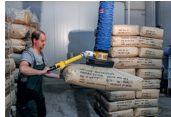
VacuPowerLift VPL-60KG Vacuum tube lifter for handling two-ply paper bags.
