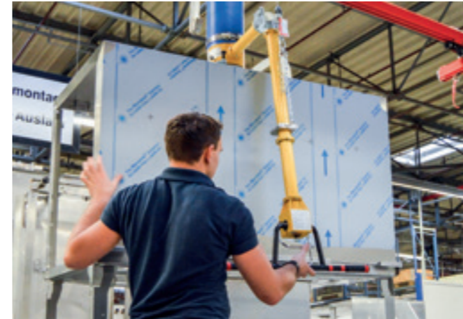
VacuPowerLift VPL-60KG Vacuum tube lifter with swivelling operating handle for steel boxes.
