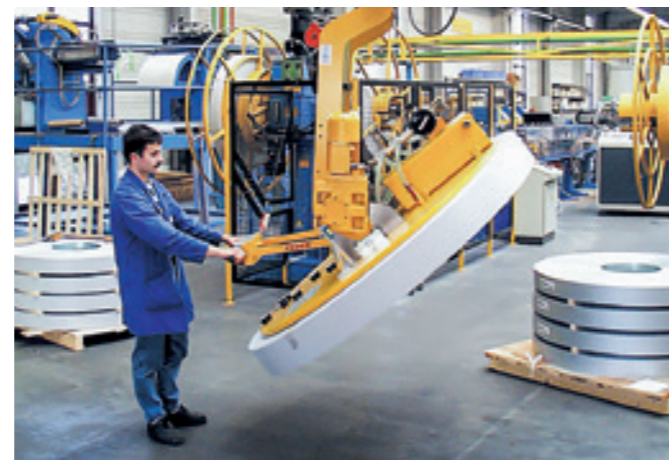
VacuCoil VC-90E-1000KG-3SK Handling slit strips for the production of roller shutter elements.
