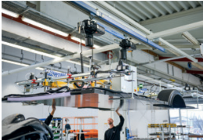
VacuBoy VB80-150KG Transport of floor elements for mobile homes with electrical lower grippers as additional security.
