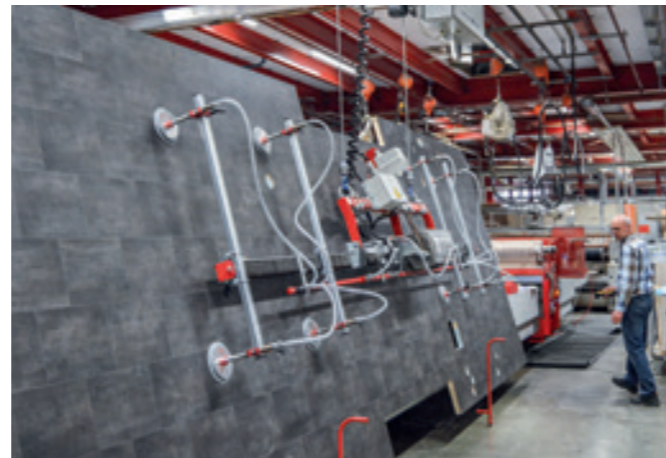
VacuBoy VB-90E-250KG Lifting unit with crane system for handling floor elements.
