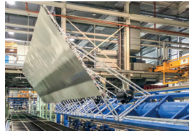
VacuStation SWS-180E-250KG Stationary turning station for sheet metal in the production of 13,000 mm-long truck sides and roof elements.
