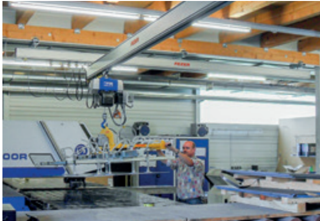
Aluminium overhead conveyor system HBS-EB-250KG With single bridge and chain hoist for handling steel sheets.
