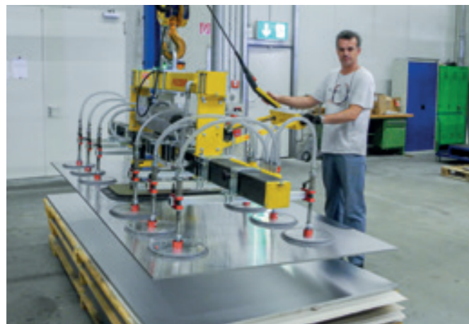
VacuBoySystem VBS-3000KG System construction cross beam for moving large steel sheets up to 6,000 mm in length.
