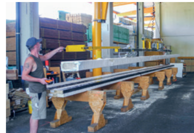
VacuWood VWLB-500KG Handling of foil-wrapped glue binders up to 12,000mm in length.
