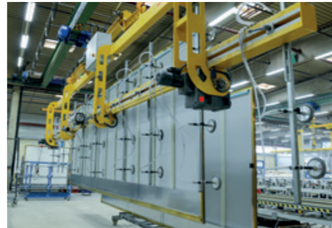
VacuGiant VG-90E-2500KG Vacuum lifter that can be swivelled by an electric motor for sandwich elements up to 12,000 mm in length.
