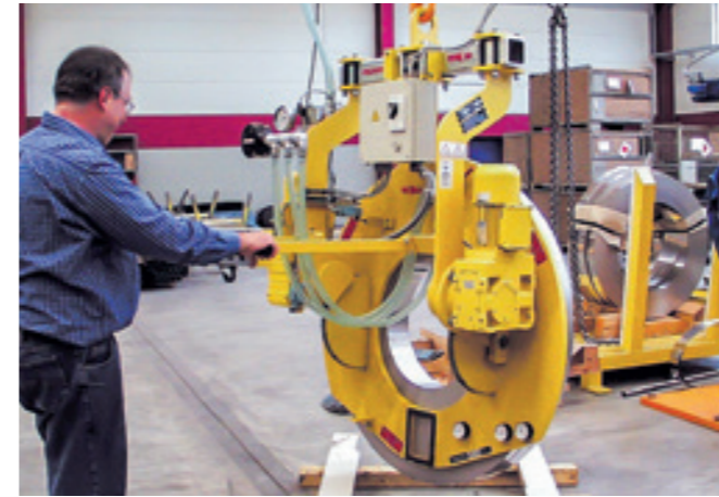
VacuCoil VC-90E-750KG-4SK Handling of aluminium split strips for the loading of punching machines.
