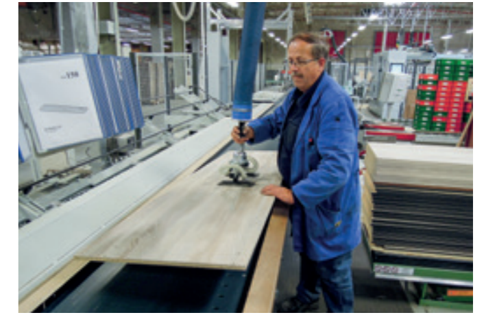
VacuQuickLift VQL-45KG Moving blockboards using a vacuum tube lifter.
