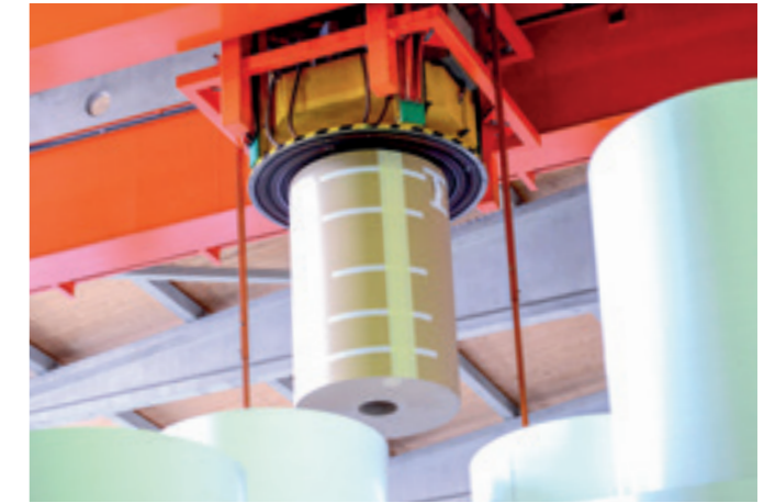
VacuCoilPaper VCP-5000KG-6SK cross beam on an automatic crane for picking paper rolls.
