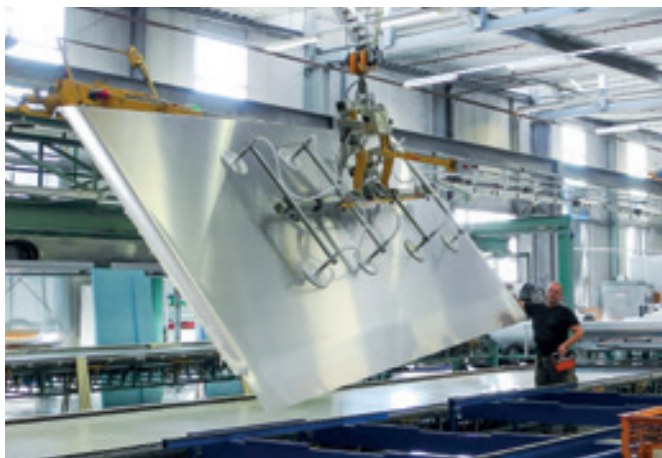
VacuBoy VB-90E-250KG Swivelling vacuum unit for handling large-format sheet metal.
