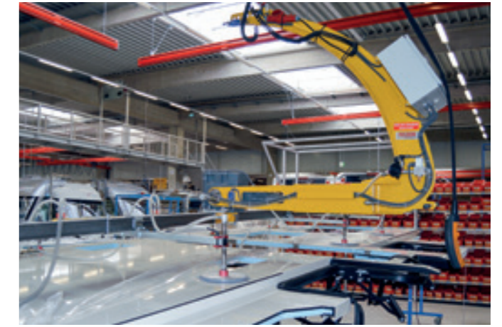
VacuBoy VB-180E-250KG Turning mobile home roofs in preassembly.
