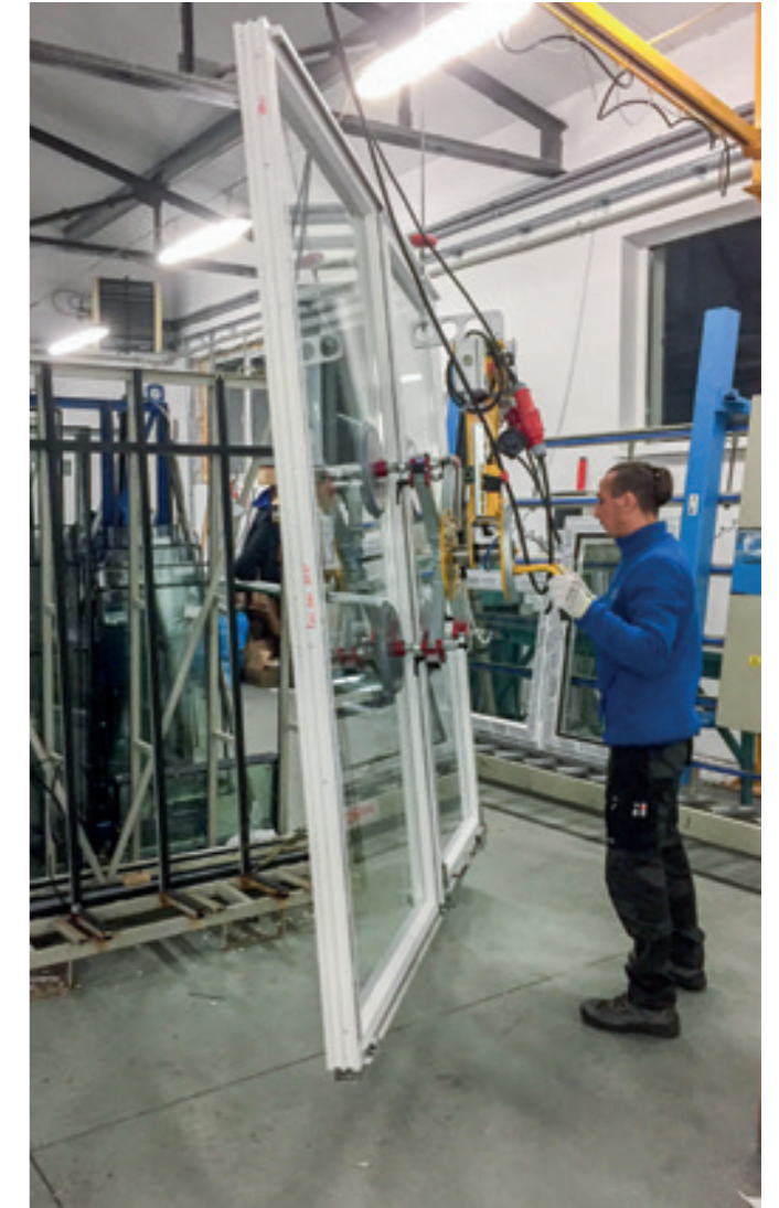
VacuBoyWindow VBW-125KG Vertical glass lifter for moving and rotating window elements.
