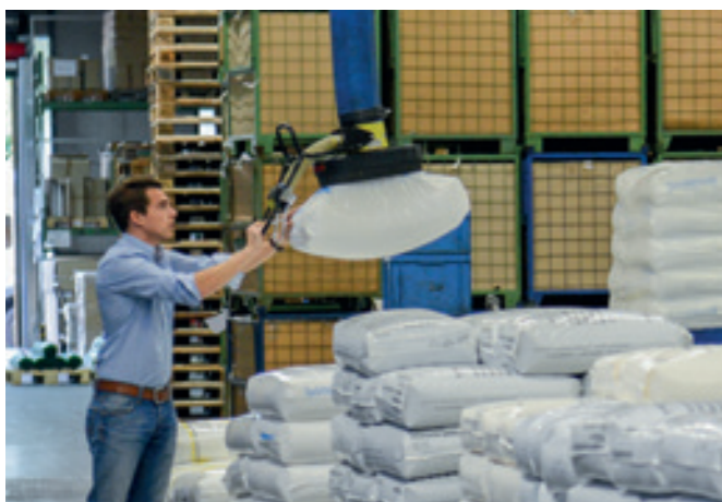
VacuPowerLift VPL-60KG Handling plastic bags.
