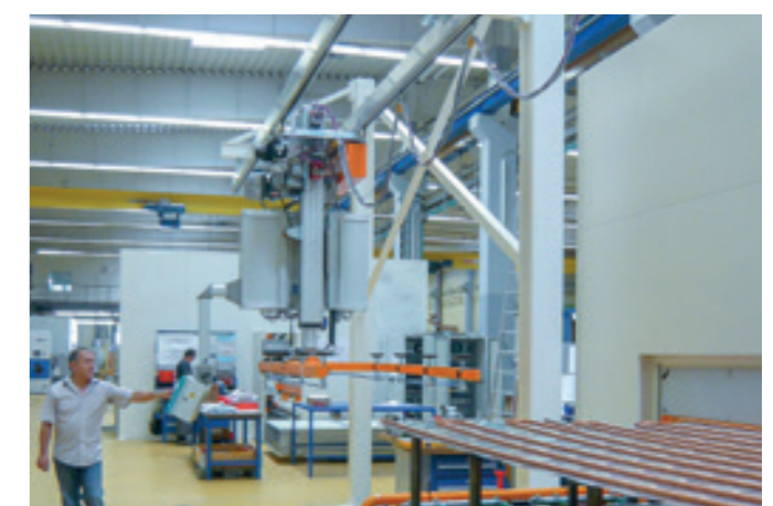
Aluminium overhead conveyor system HBS-DB-LF-100KG with steel construction, rigid lifting system and electric friction wheel drive in semi-automatic operation.
