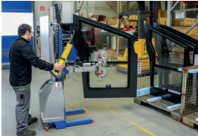
MobilLift ML-90E-45KG Mobile working stand with electric swivel mechanism for window elements.
