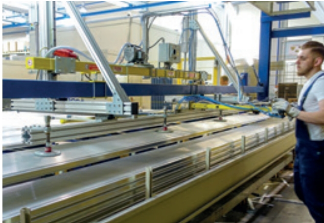
LiftFix LF-125KG Pneumatically controlled, rigid lifting system for feeding aluminium profiles to a punching machine.
