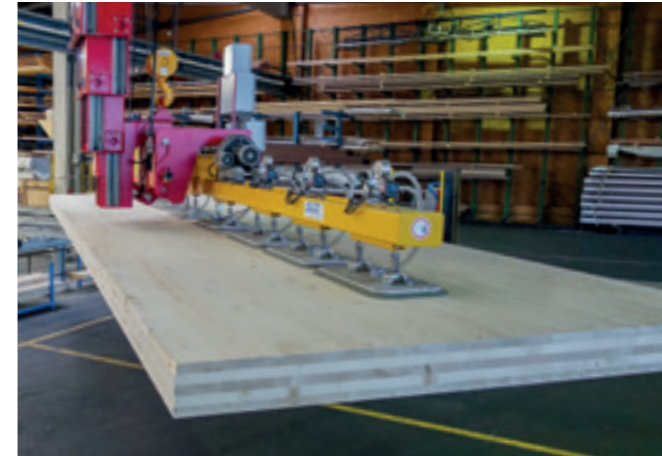
VacuPoro VP-3000KG Vacuum lifter on a rigid lifting axis for handling massive solid wood panels.
