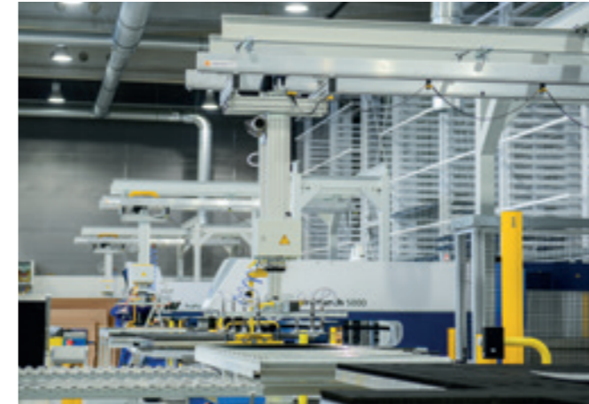
LiffFix LF-250KG Several rigid stroke guidance systems for the precise positioning of steel sheets on laser cutting systems.
