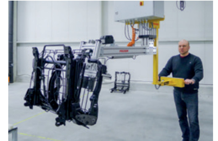
LiffFix LF-100KG LiffFix rigid lifting system for handling steel seating groups for preassembly.
