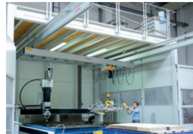
Aluminium overhead conveyor system HBS-EB-250KG with single bridge and cantilever steel structure for support-free removal of components.
