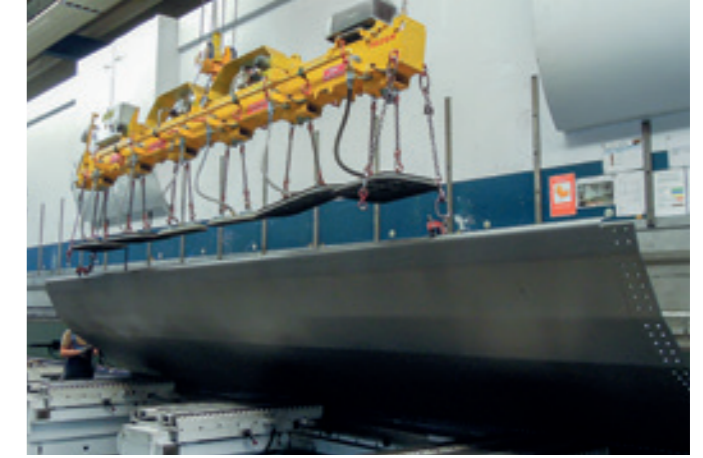
VacuGiantVario VGV-6000KG Vacuum cross beam on an edging machine to support the sheet metal upstand.
