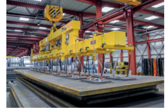
VacuGiant VG-25000KG Heavy-duty cross beam for the horizontal handling of large-format sheet metal up to 16,000 x 3,500 x 300 mm.
