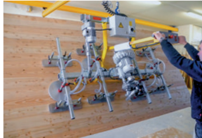
VacuPoro VP-90E-250KG Swivel-action lifting device for handling blockboard and chipboard.
