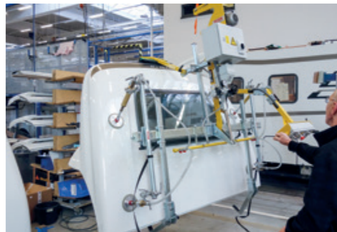
VacuBoy VB-90E-150KG Handling alcove structures through 90°.
