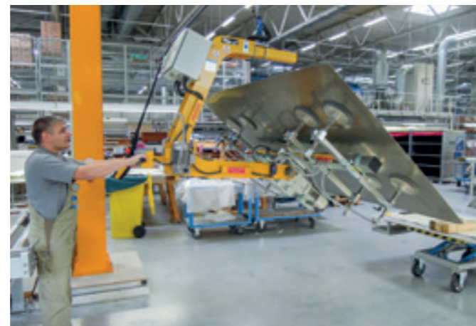
VacuBoy VB-180E-250KG 180° turning unit for sheet steel.
