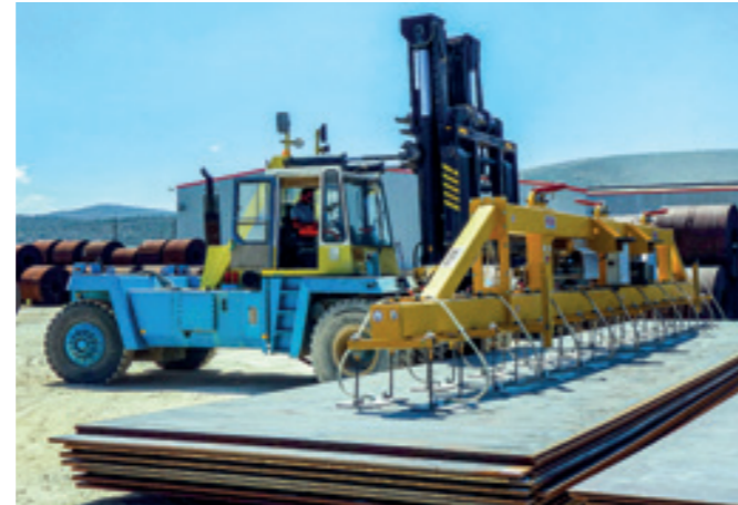
VacuGiant VG-SG-12000KG Vacuum cross beam for forklift operation outdoors with a heating system and its own power generator.
