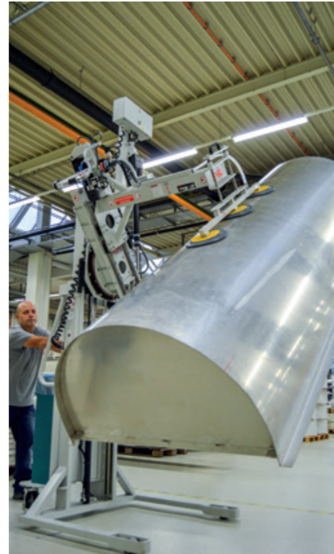
MobiLift ML-180E-250KG With electrical lifting and swivel unit for handling moulded elements.
