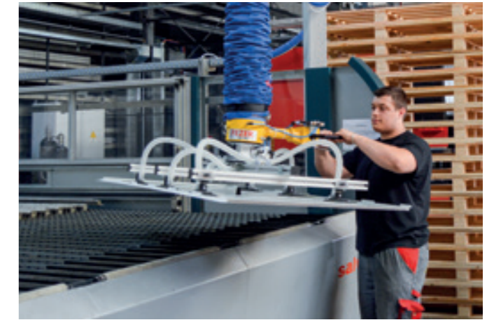
VacuPowerLift VPL-80KG Vacuum tube lifter for feeding sheet metal to a laser cutting system.
