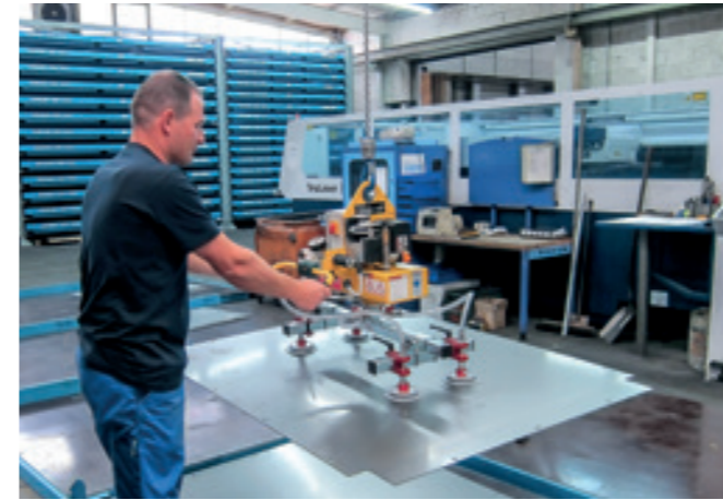
VacuBoyMini VBM-ACCU-125KG Mains-independent battery-operated vacuum lifter for small-format sheets.
