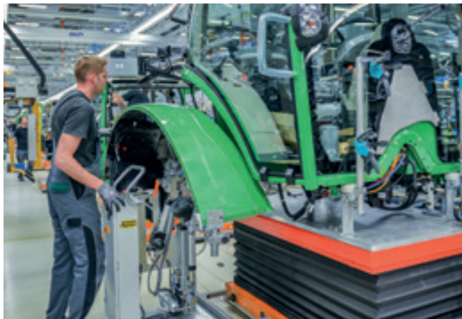
VacuStand VS-I-125KG Mobile working stand for docking and final assembly of fenders on an AGV station.
