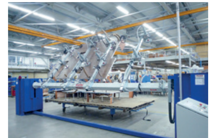
VacuStation SWS-180E-250KG Stationary turning system with electrical height adjustment for mobile home floor elements.
