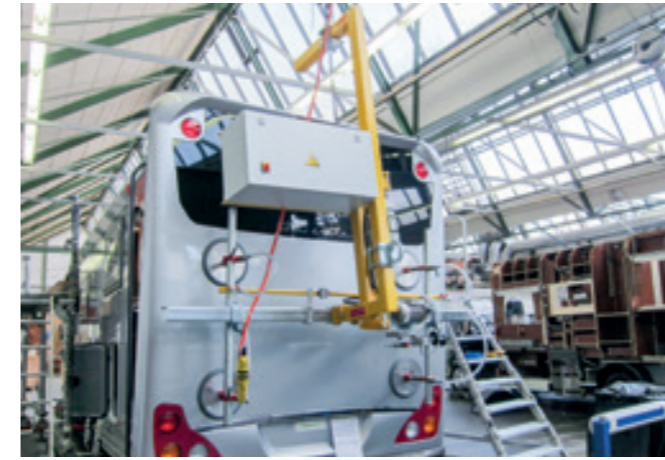
VacuBoy VB-VERT-250KG Vertical handling of rear wall elements in final assembly.
