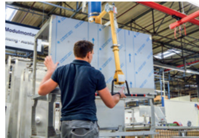
VacuPowerLift VPL-80KG Handling of large sheet metal housings with a tube lifter with crankable handle.
