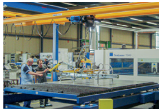
Steel overhead conveyor system HBS-EB-500KG Double bridge with a span of 8,000 mm, chain hoist and vacuum lifter.
