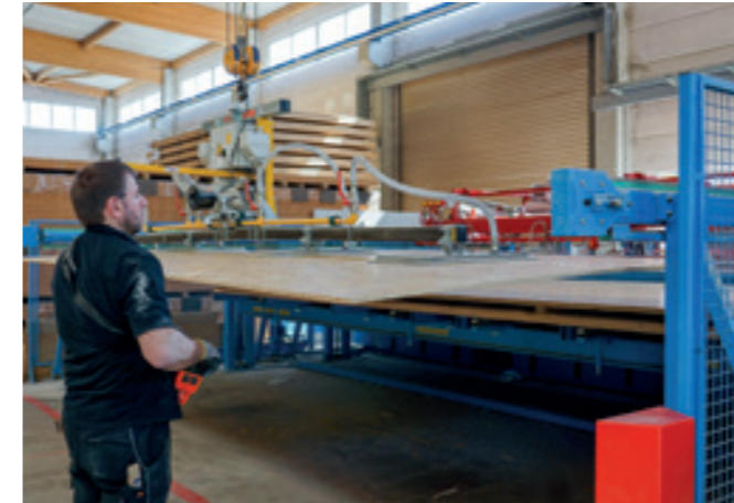
VacuPoro VP-90E-500KG Swivel-action lifting unit for loading a CNC woodworking system.
