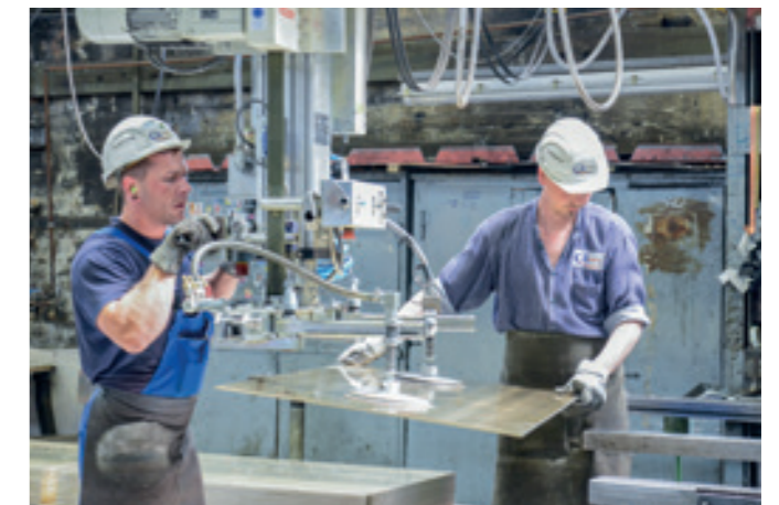
LiftFix LF-250KG Rigid lifting system with slewing ring for loading an edge press with copper sheets.
