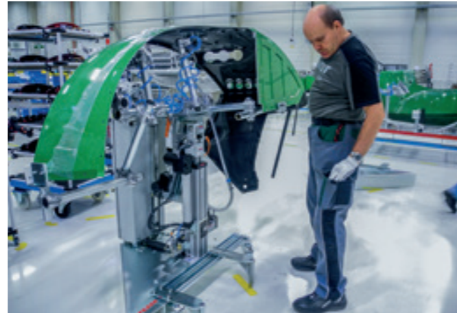
VacuStand VS-I-125KG Mobile working stand for the preassembly of fenders for tractors.
