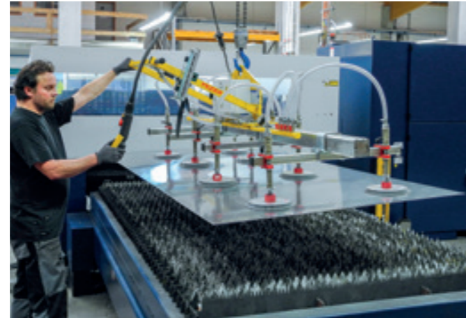
VacuBoy VB-500KG Vacuum lifter for loading a laser cutting system with large-format sheets.
