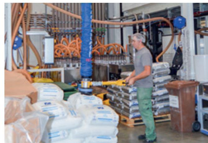
VacuPowerLift VPL-60KG Tube lifter with an articulated operating handle for handling plastic bags.
