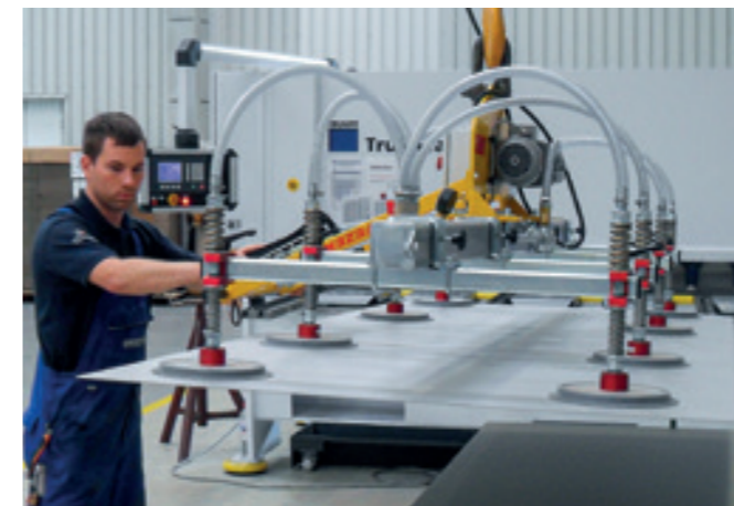
VacuBoy VB-1000KG Handling large-format sheets on a nipple machine.
