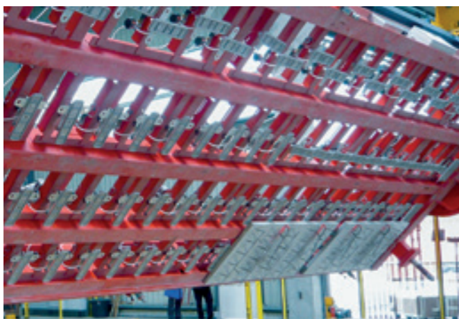
VacuStation SWS-2500KG Loading stone slabs into a wet grinding machine using a battery-operated vacuum lifter.
