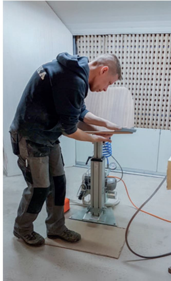
VacuStand VS-60KG With manual lifting, turning and swivel unit for working on seat chairs.
