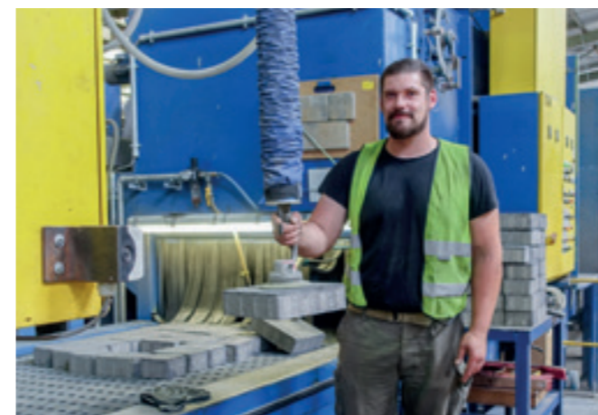
VauQuickLift VPQ120-40KG Handling paving stones using a vacuum tube lifter.
