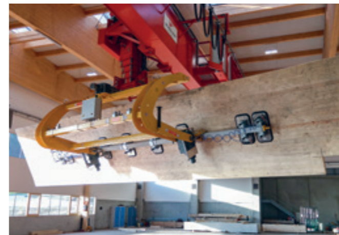
VacuPoro VP-180E-1000KG Vacuum lifter for turning solid wood panels 8,000 mm in length.
