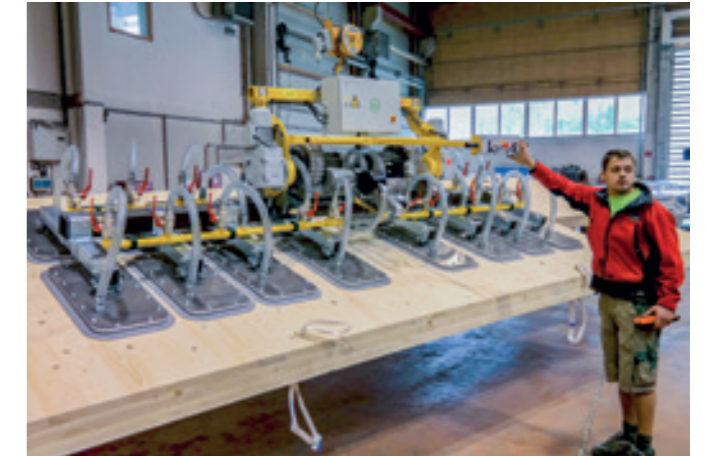
VacuPoro VP-90E-1500KG Vacuum lifter for swivelling solid wood panels 8,000 mm in length.
