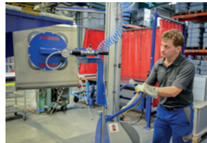
Mobilift ML-60KG Mobile variable-height working stand for feeding sheet metal parts to a welding station.
