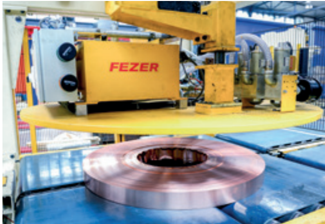
VacuCoil VC-1500KG-4SK Coil suction plate in Automatic mode for copper slit strip rings.
