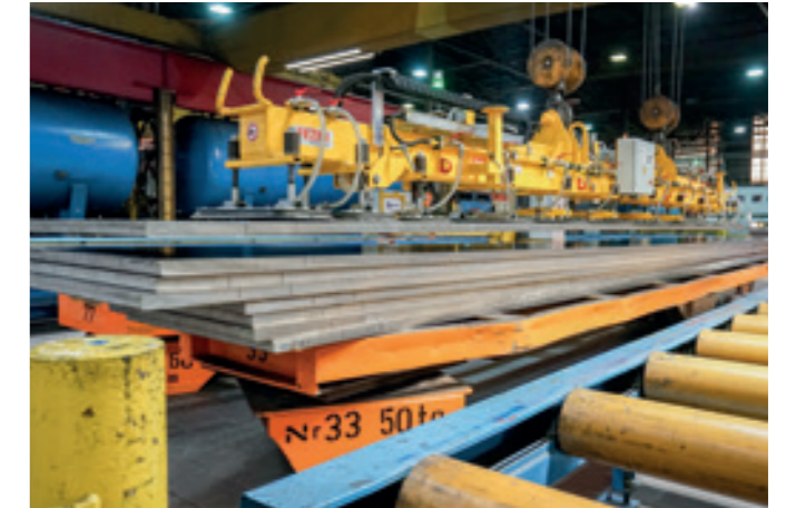
VacuGiant VG-TEL-8000KG Manually telescopic vacuum cross beam for moving aluminium sheets of up to 14,000 mm in length.
