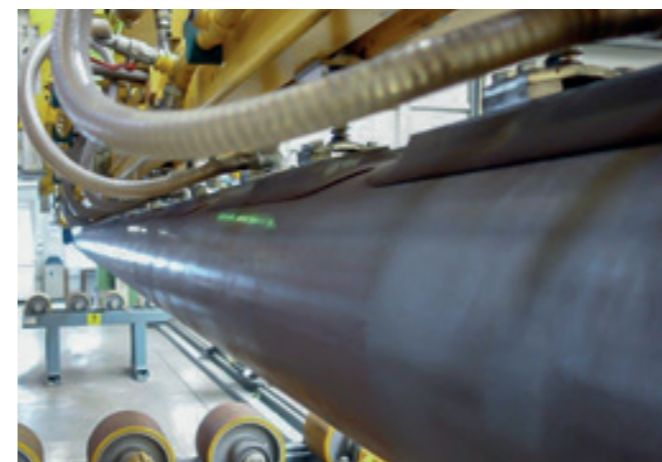
Vacuum Lifting Device VLM-3000KG Vacuum cross beam on an automatic crane for pipes up to 6,000 mm in length.
