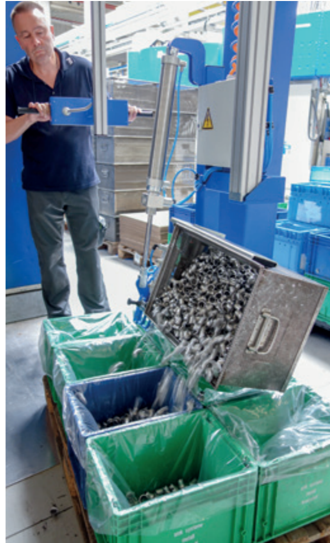
LiftFix LF-1200-60KG Rigid lifting system with pneumatic swivel unit for emptying small mesh boxes.
