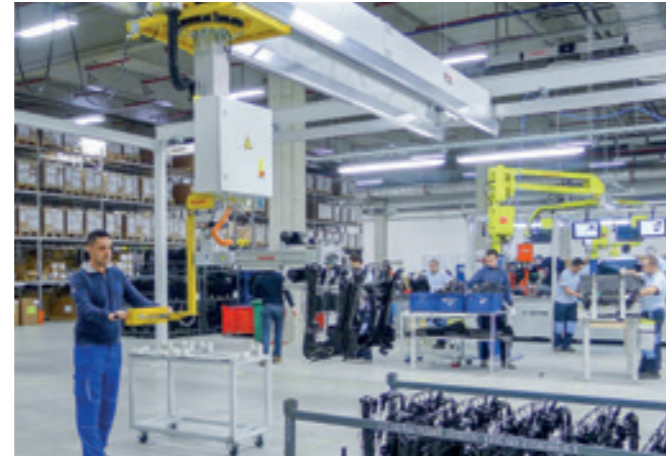
Aluminium overhead conveyor system HBS-DB-125KG With double bridge and rigid Liffix lifting system for moving seat frames.
