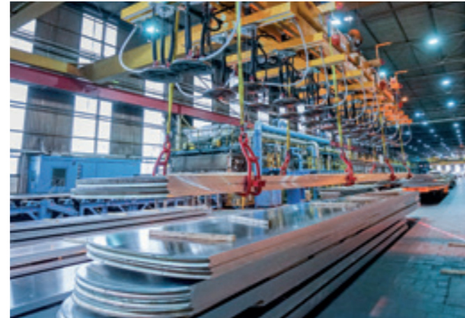
VacuGiant VG-TEL-6000KG For single transport or multi-layer transfer of aluminium plates with vacuum or gripping hook.
