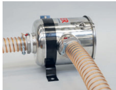
Vacuum filter and antistatic tubes Made of stainless steel with electrically connected filter insert and antistatic feed tubes, which are electrically conductively connected to the assembly units.
