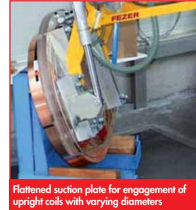
Flattened suction plate for engagement of upright coils with varying diameters
