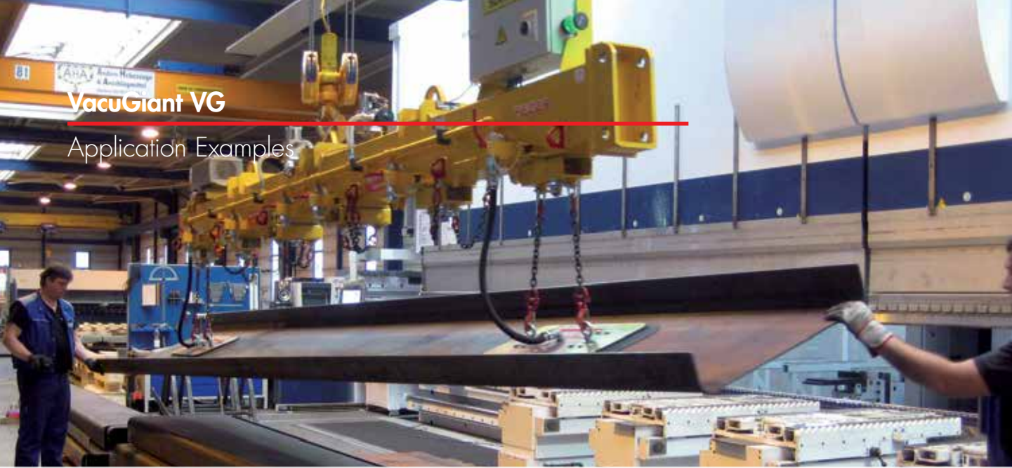
VacuGiant on a bending machine with chain suspension
