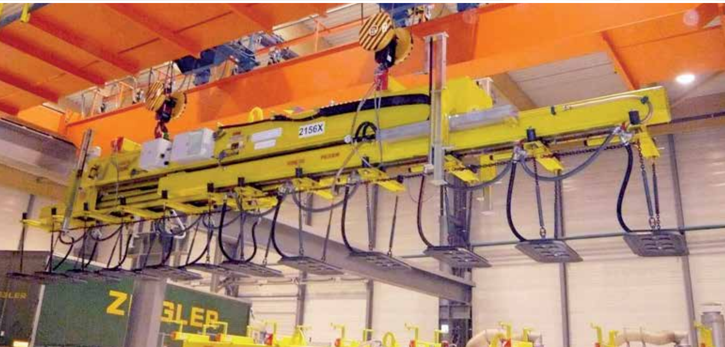
VacuGiant with 12.000 kg carrying capacity and electrically extendable main beam from 8 to 12 m
